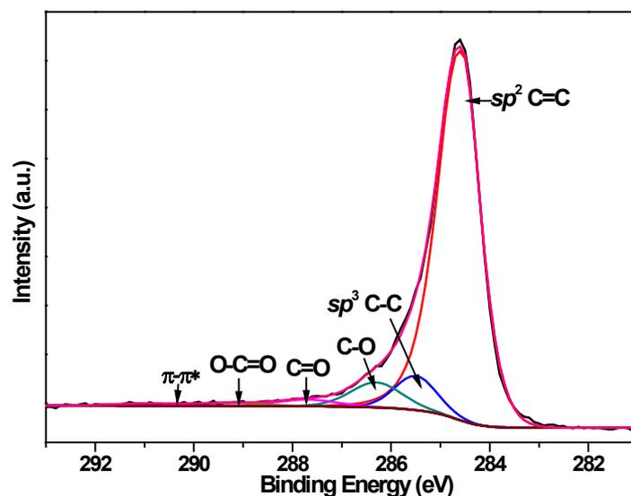
**Figure S5.**  $\text{C}1\text{s}$  XPS spectrum, analyzed in components corresponding to the graphene sheets and the oxygen containing species
