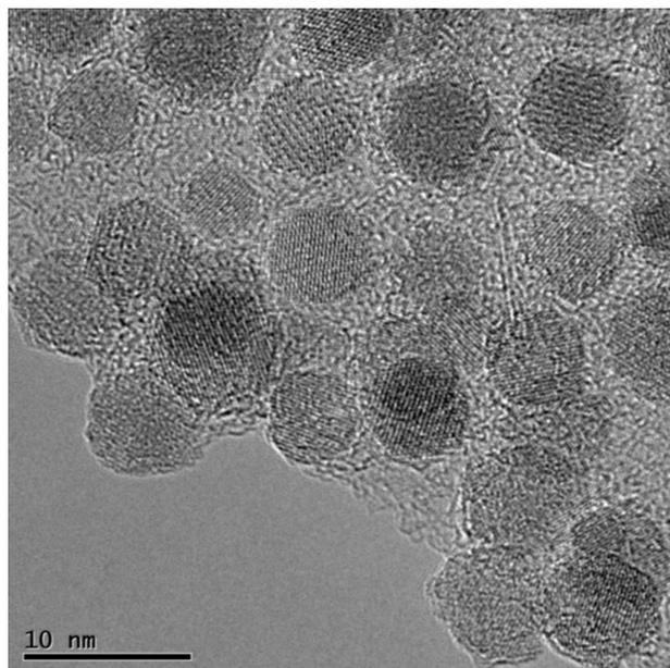
**Figure S8.** TEM images at different magnifications of  $\text{Fe}_3\text{O}_4$  NPs *homogeneously and densely packed on the multivalent platform His<sub>6</sub>@GN* obtained by assisted-exfoliation of expanded graphite by  $\text{NH}_2\text{-His}_6\text{-pyrene 1}$ .
