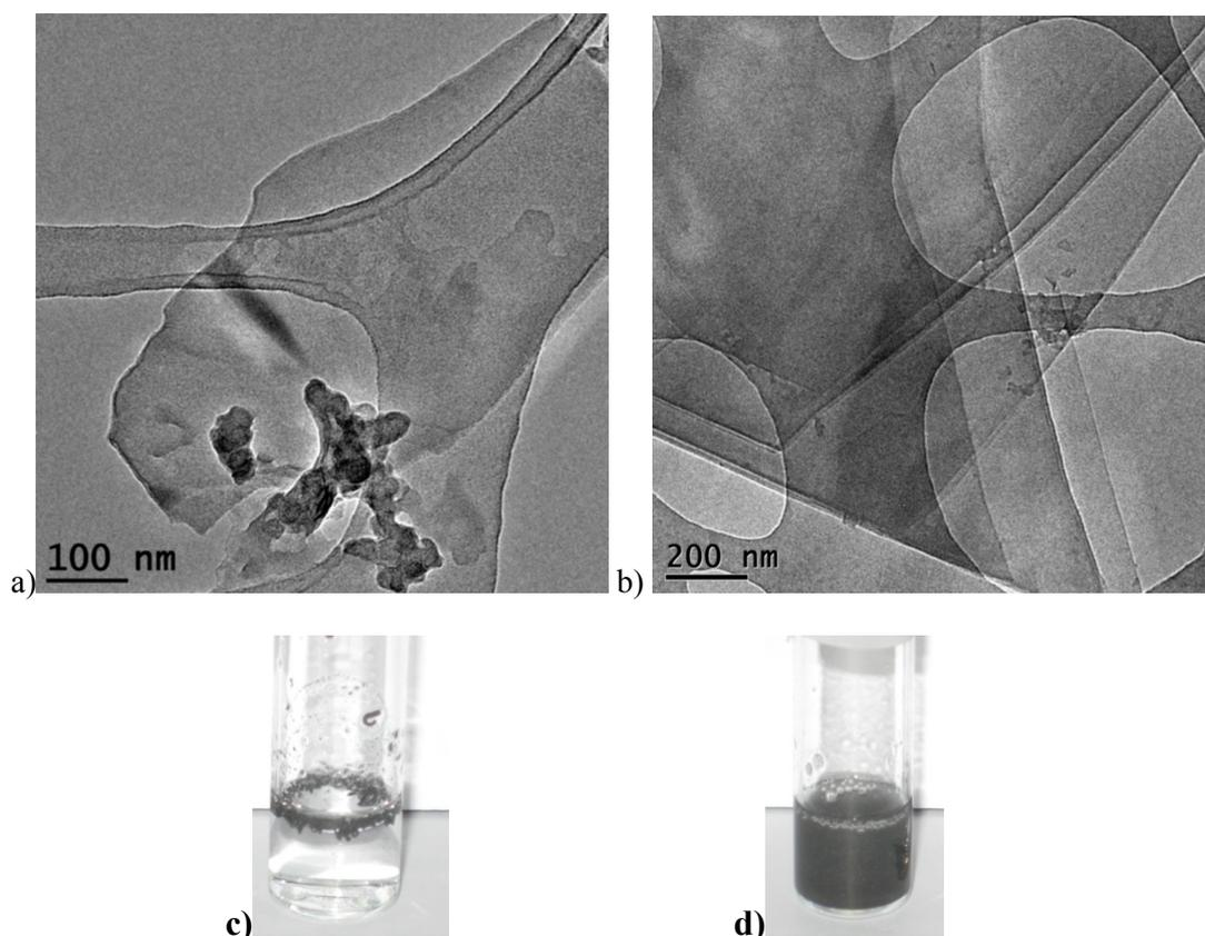
**Figure S1.** *Top*: TEM images recorded on typical fragments obtained by: a) simple sonication of expanded graphite without amphiphilic molecule; b) assisted-exfoliation of expanded graphite by NH<sub>2</sub>-His<sub>6</sub>-pyrene. *Bottom*: optical images of the samples containing the solution; c) non functionalized expanded graphite in water, d) stable colloidal dispersion of His<sub>6</sub>@GN.
