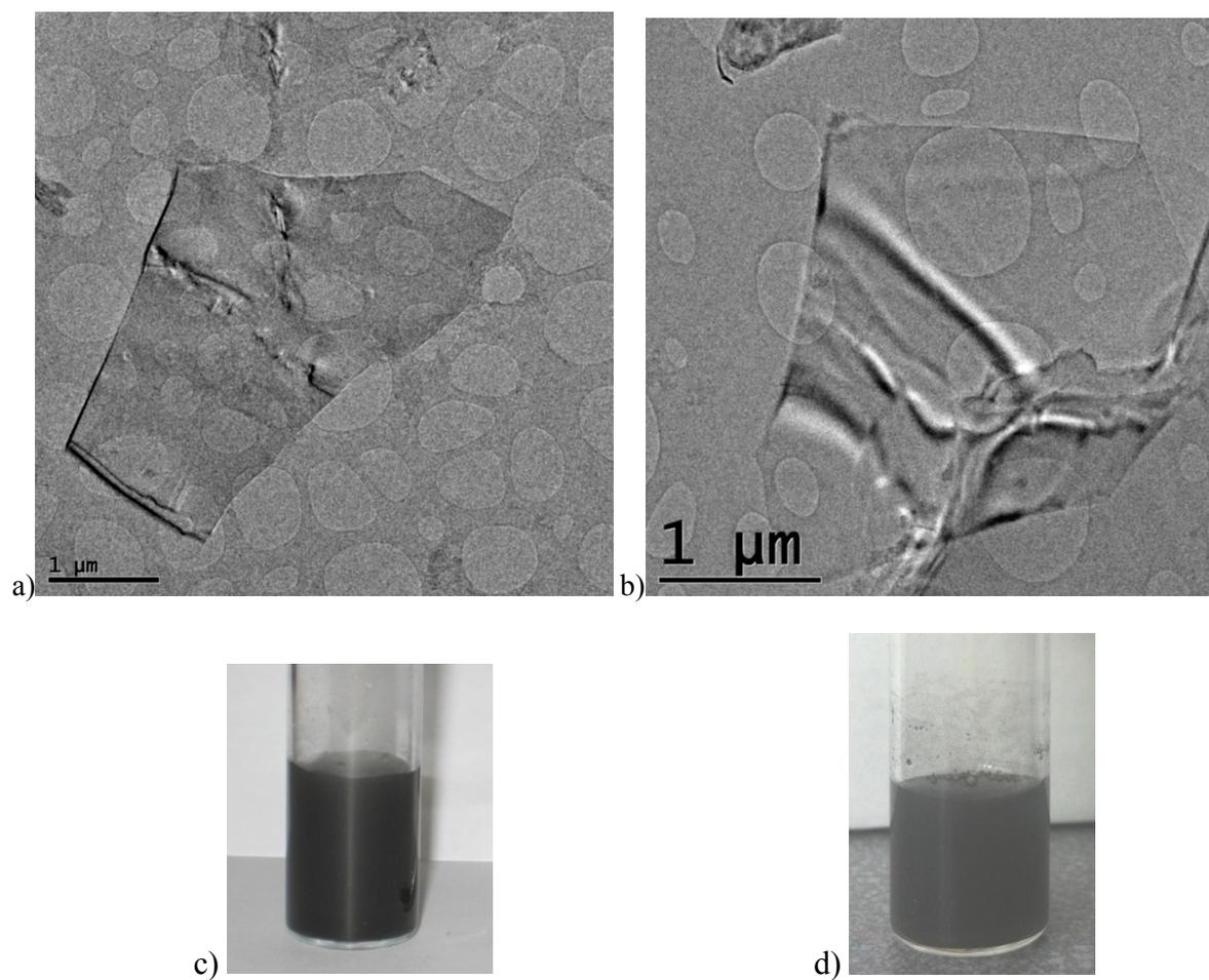
**Figure S2.** TEM (a) and b)) and optical images (c) and d)) of representative His<sub>6</sub>@GN obtained by assisted-exfoliation of expanded graphite by NH<sub>2</sub>-His<sub>6</sub>-pyrene as-prepared (left) and after 6 months of another sample (d) prepared in the same manner (right), respectively.
