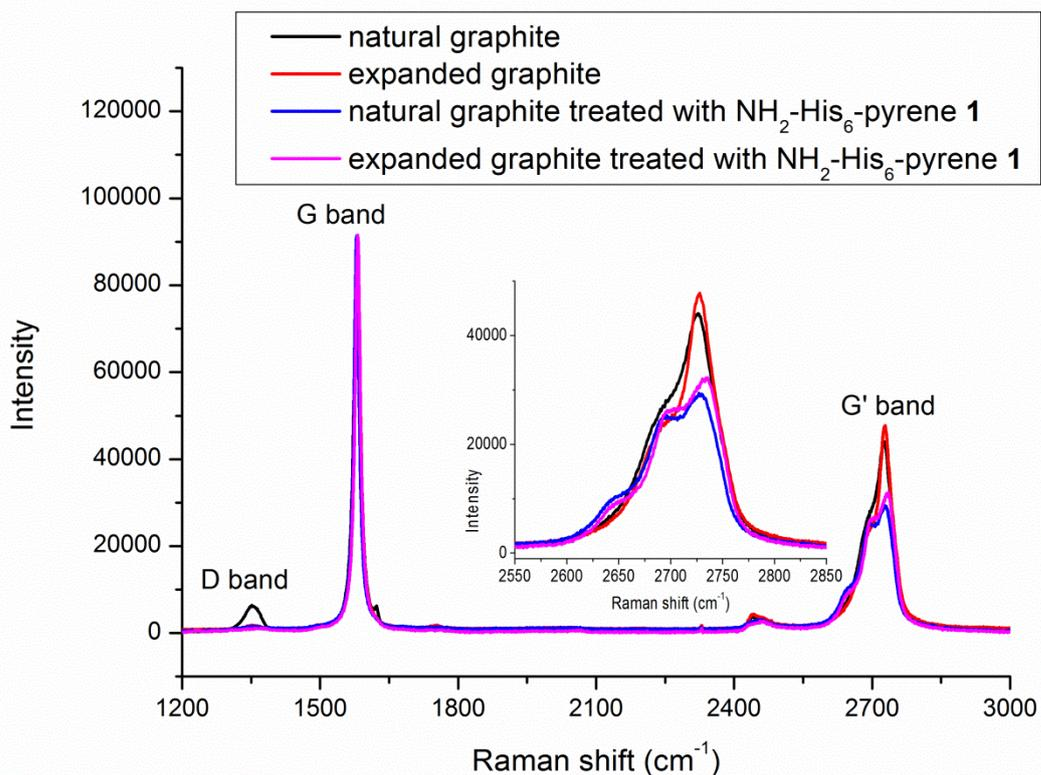
**Figure S4 :** Full Raman spectra of the natural and expanded graphite samples before and after treatment with peptides (414 nm excitation).
