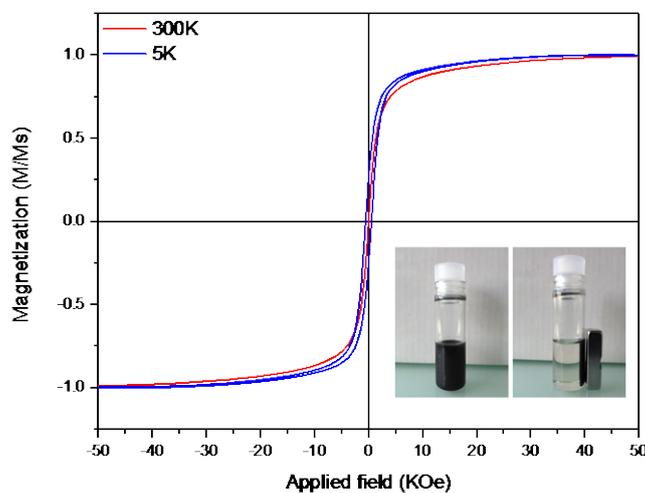
**Figure S9.** Magnetization curves of nanoparticles NPs/FLG as a function of applied magnetic field at 300 K and 5 K. Inset: Magnetic interaction between the NPs/FLG sample and the external magnet allowing the easy separation of the solid from the solution.
