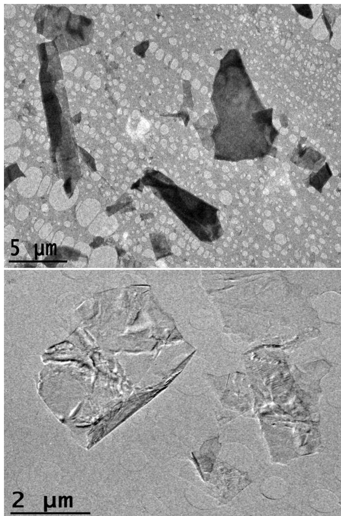
**Figure S3.** TEM images at different magnifications of His<sub>6</sub>@FLGs obtained by assisted-exfoliation of expanded graphite by NH<sub>2</sub>-His<sub>6</sub>-pyrene **1**.
