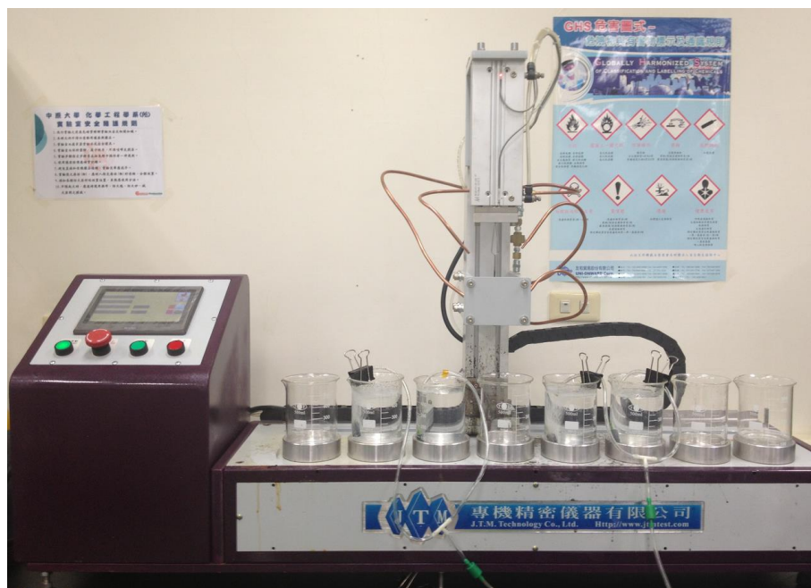
Fig. S1. Homebuilt robotic dipping machine.
