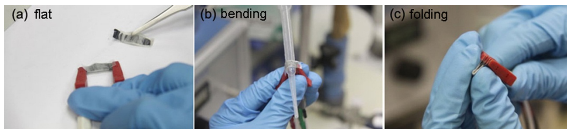
Figure S7. Photographs of the assembled rectangular shape supercapacitors fabricated using SWCNT–MnO 2 –paper composites under different bending test conditions. (a) flat, (b) bending at 90°, and folding of 180°.
