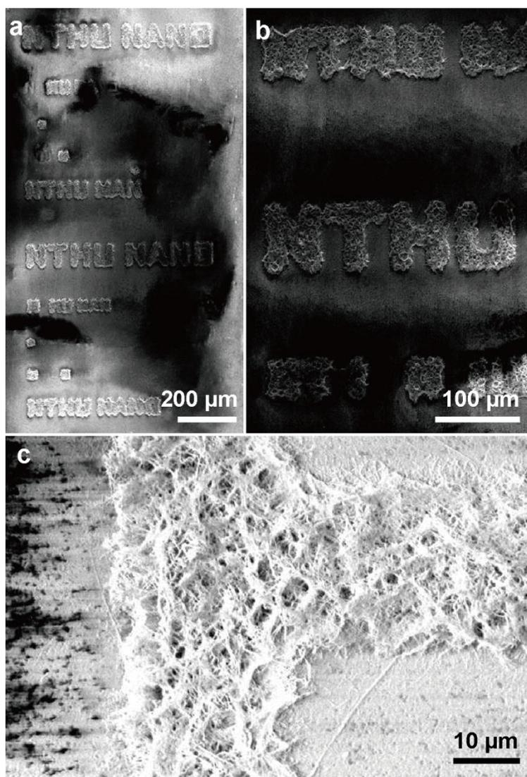
**Fig. S5.** SEM images of  $\text{Cu}_3\text{Si}$  nanowires grown on a Cu-patterned substrate.
