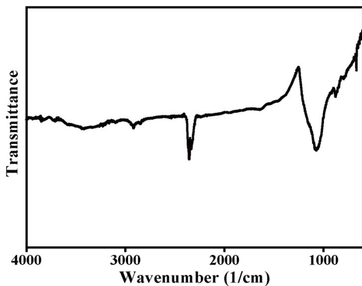
Fig. S3. FTIR spectrum of  $\text{Cu}_3\text{Si}$  nanowires.
