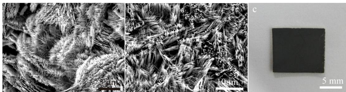
**Fig. S1.** (a-b) top-view SEM images of Cu<sub>3</sub>Si nanowires grown on a Cu substrate obtained from the reaction by decomposition of monophenylsilane at 495 °C, 10.3 MPa at supercritical hexane. (c) Photograph of the Cu substrate after a reaction.
