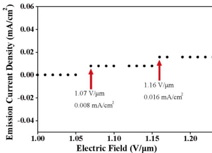
Fig. S4. Field emission profile of arrayed  $\text{Cu}_3\text{Si}$  nanowires extracted from Fig. 7, at the region that the electric field ranges from 1.00 to 1.20  $\text{V}/\mu\text{m}$  and emission current density ranges from 0.00 to 0.06  $\text{mA}/\text{cm}^2$
