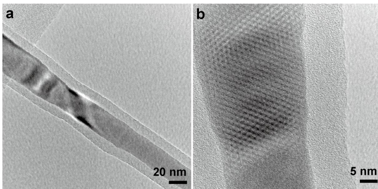
**Fig. S2.** TEM images of a Cu<sub>3</sub>Si nanowire.
