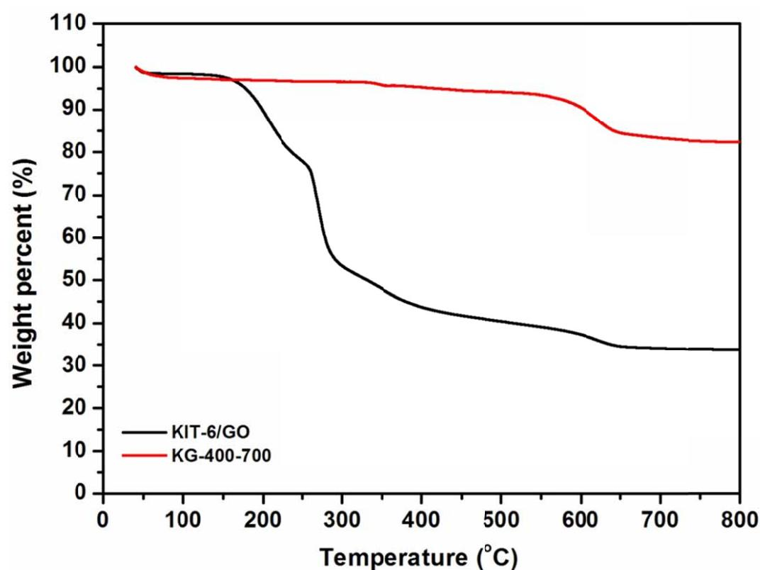
**Figure S3.** TGA plots of KIT-6/GO and KG-400-700 obtained at  $10 \text{ mLmin}^{-1}$  air flow and a heating rate of  $10 \text{ }^{\circ}\text{Cmin}^{-1}$ .
