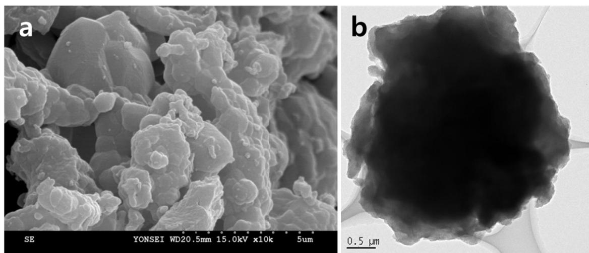
**Figure S4.** (a) SEM and (b) TEM image of KIT-6.
