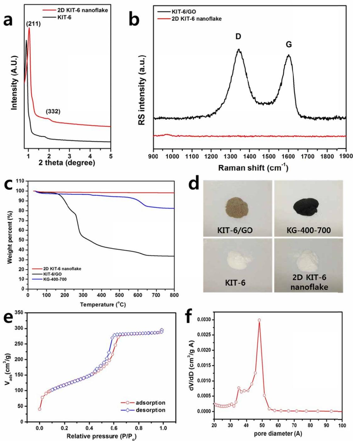
**Figure S5.** (a) Low angle XRD pattern of KIT-6 and 2D KIT-6 nanoflake (b) Raman spectra of KIT-6/GO and 2D KIT-6 (c) TGA plots of KIT-6/GO, KG-400-700 and 2D KIT-6 nanoflake (d) photographic image of KIT-6/GO, KG-400-700, KIT-6, and 2D KIT-6 nanoflake powder (e)  $\text{N}_2$  adsorption isotherms and (f) pore size distribution of 2D KIT-6 nanoflake.
