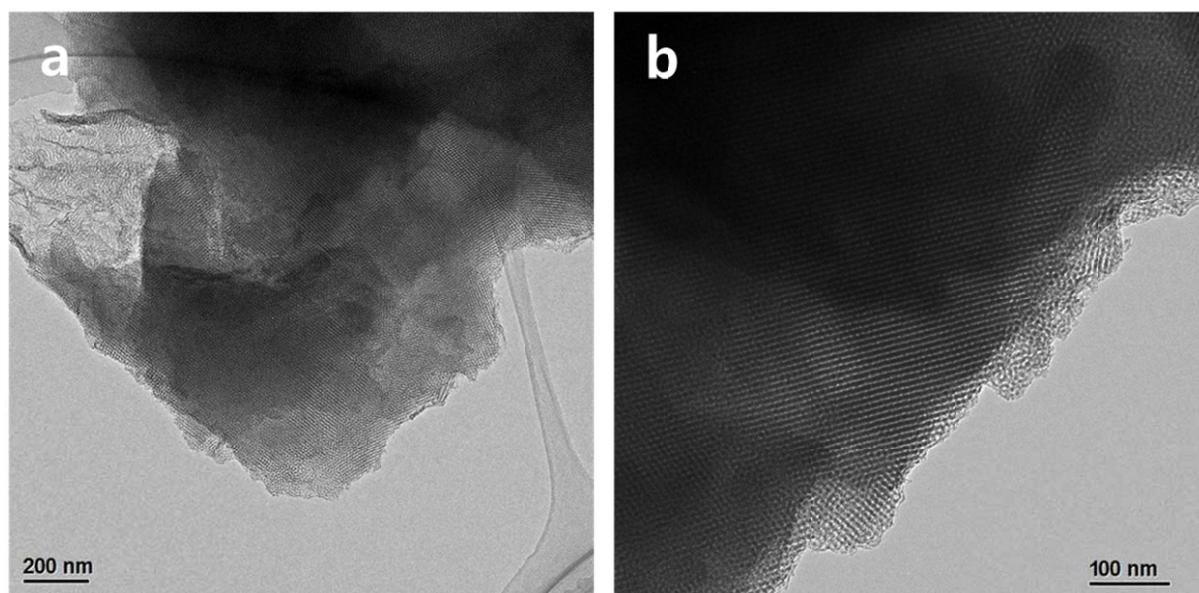
**Figure S2.** Typical TEM image of (a) KIT-6/GO nanocomposite and (b) HRTEM image of KIT-6/GO nanocomposite.
