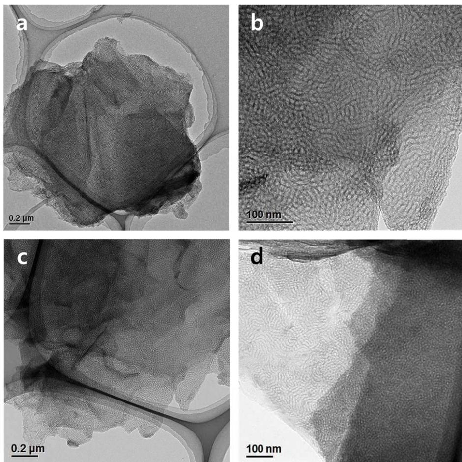
**Figure S1.** Typical TEM images of disordered mesoporous silica/graphene nanocomposite with different loading amount of (a-b) 66 wt.% and (c-d) 50 wt.%.
