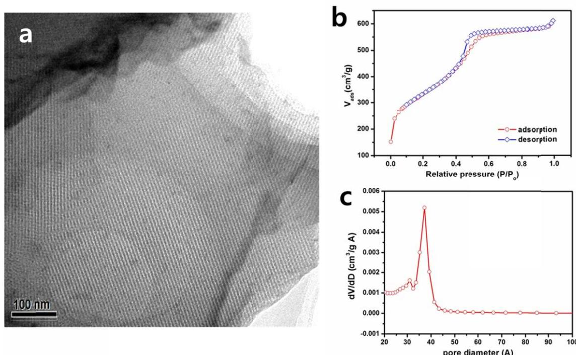
**Figure S6.** (a) Typical TEM image of mesoporous carbon/graphene composite material (b)  $\text{N}_2$  adsorption isotherms and (c) pore size distribution of mesoporous carbon/graphene composite material.
