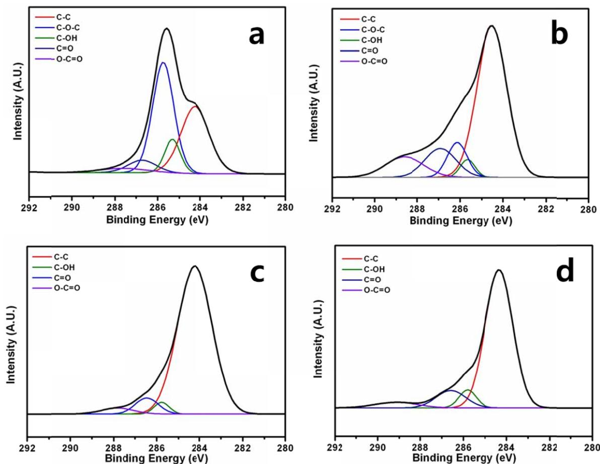
**Figure S7.** XPS C1s spectra of (a) KIT-6/GO, (b) KG-400, (c) KG-400-700 and (d) KG-700.
