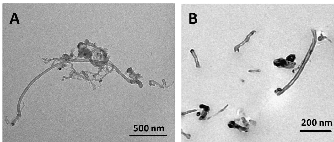
**Figure S2.** TEM images of MWCNT-NH<sub>3</sub><sup>+</sup>. Multi-walled CNTs are clearly present as individualized entities. A) These nanotubes were dispersed in 5% dextrose and deposited on the TEM grid and dried before observation. B) These nanotubes were prepared as described in the Experimental Section, under transmission electron microscopy studies, by the same method applied to prepare the cell cultures for TEM imaging.
