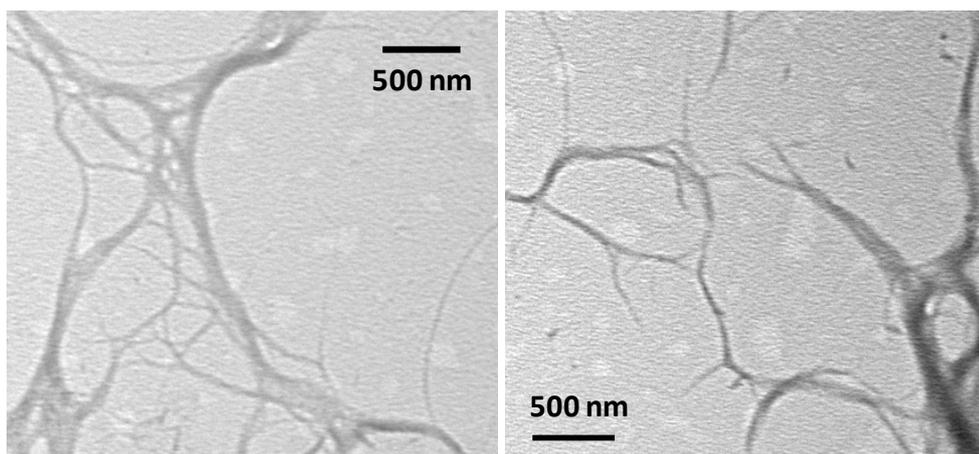
**Figure S1.** TEM images of SWCNT-NH<sub>3</sub><sup>+</sup>. Single-walled CNTs have always the tendency to re-bundle when deposited in the TEM grid during solvent evaporation. It is not possible in this case to evidence the presence of isolated tubes.
