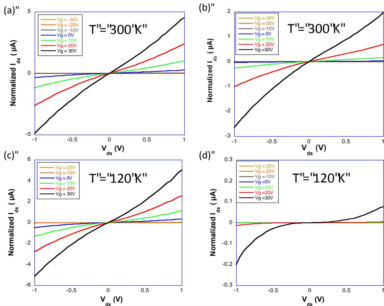
**Fig. S2** Room temperature  $I_{ds}$ - $V_{ds}$  characteristics for the MoS<sub>2</sub> devices on (a) h-BN and (b) SiO<sub>2</sub> substrate. Low temperature  $I_{ds}$ - $V_{ds}$  characteristics at  $T = 120$  K for the MoS<sub>2</sub> devices on (c) h-BN and (d) SiO<sub>2</sub> substrate.
