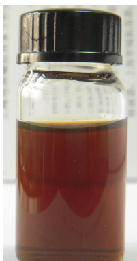
Figure S1. Typical digital photograph of 1 mg/mL GO suspension.
