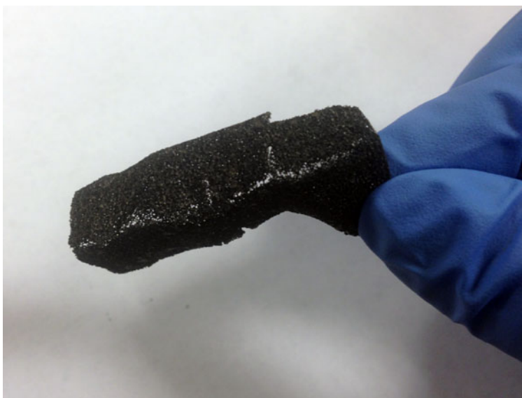
Figure S3. Digital picture shows the structurally collapsed rGO-8-Ni foam. rGO-Ni electrodes became fragile after repeating the loading process for 6 times or above due to the chemical dissolution of nickel in acidic GO aqueous solution (pH ~5)
