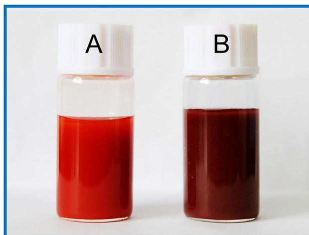
**Fig.S6** Digital photos of suspension of (A) pure dendritic  $\alpha$ -Fe<sub>2</sub>O<sub>3</sub> and (B) Au NPs grafted on dendritic  $\alpha$ -Fe<sub>2</sub>O<sub>3</sub>. It is indicated that, pure dendritic  $\alpha$ -Fe<sub>2</sub>O<sub>3</sub> is ferric oxide red while NPGDF is dark red.
