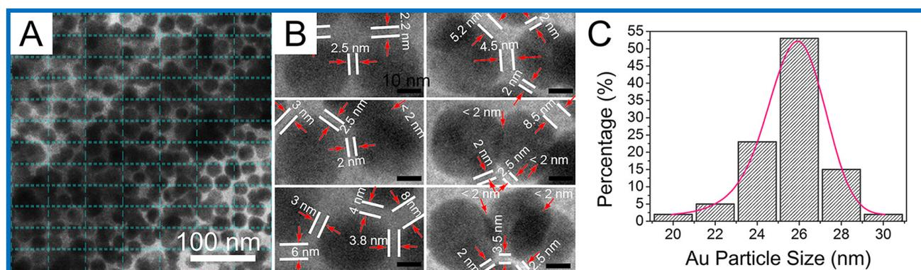
**Fig.S5** (A) Typical TEM image of NPGDF. (B) Typical higher-magnification TEM images and the specific measurements of Au NPs size and gap distance distribution of interparticle separations. (C) Au NPs size distribution. Most NPs size were about 24~28 nm with narrow size distribution.
