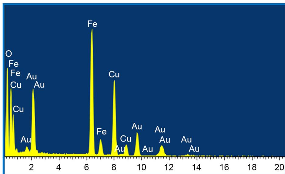
**Fig.S4** EDS spectrum of NPGDF. It is indicated that as-prepared product consists of Fe, O and Au. As a note, the Cu element was detected in the sample originate from copper grids.
