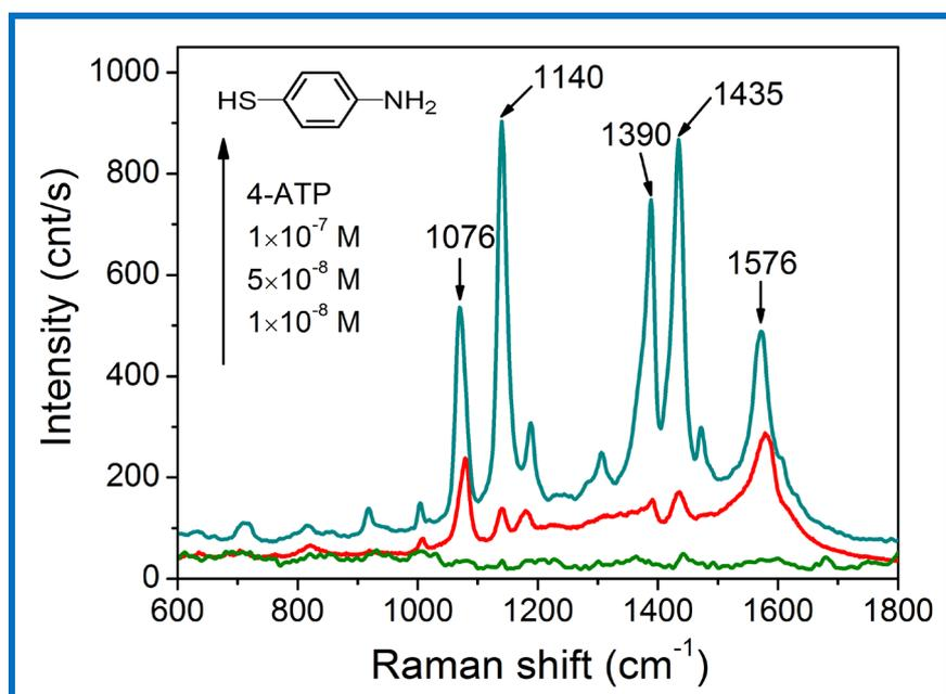
**Fig.S8** Series of SERS spectra of 4-ATP with NPGDF as SERS substrates after storing at room temperature for three months.
