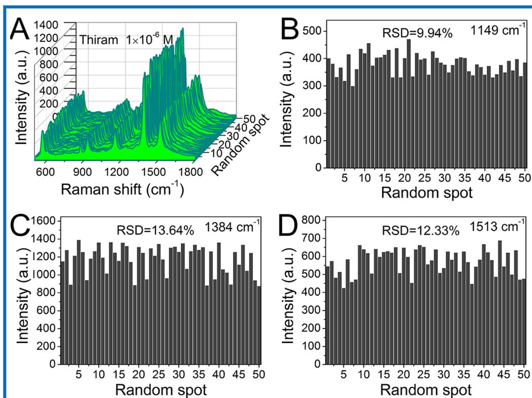
**Fig.S10** (A) Series of SERS spectra of  $10^{-6}$  M thiram collected on randomly from 50 spots of the NPGDF. (B), (C) and (D) are the intensities of the main vibrations of  $10^{-6}$  M thiram for the 1149, 1384 and 1513  $\text{cm}^{-1}$  corresponding to (A) respectively.
