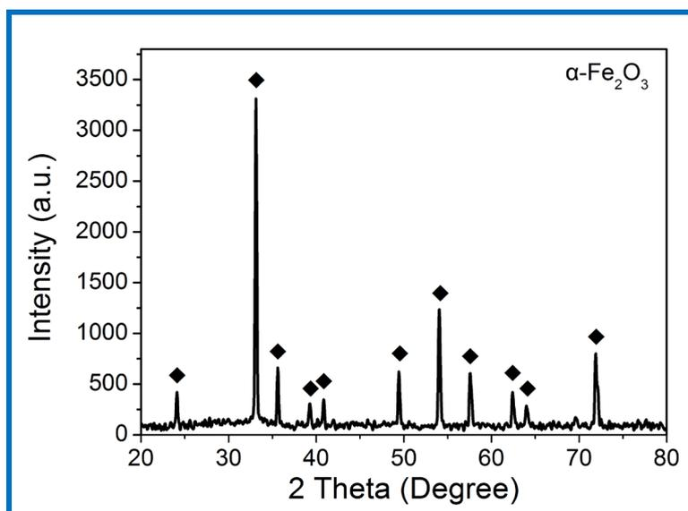
**Fig.S2** XRD patterns of as-prepared dendritic  $\alpha\text{-Fe}_2\text{O}_3$ . All of the diffraction peaks can be attributed to the  $\alpha\text{-Fe}_2\text{O}_3$  phase (JCPDS 33-0664) and the narrow sharp peaks suggest that the products are highly crystalline.
