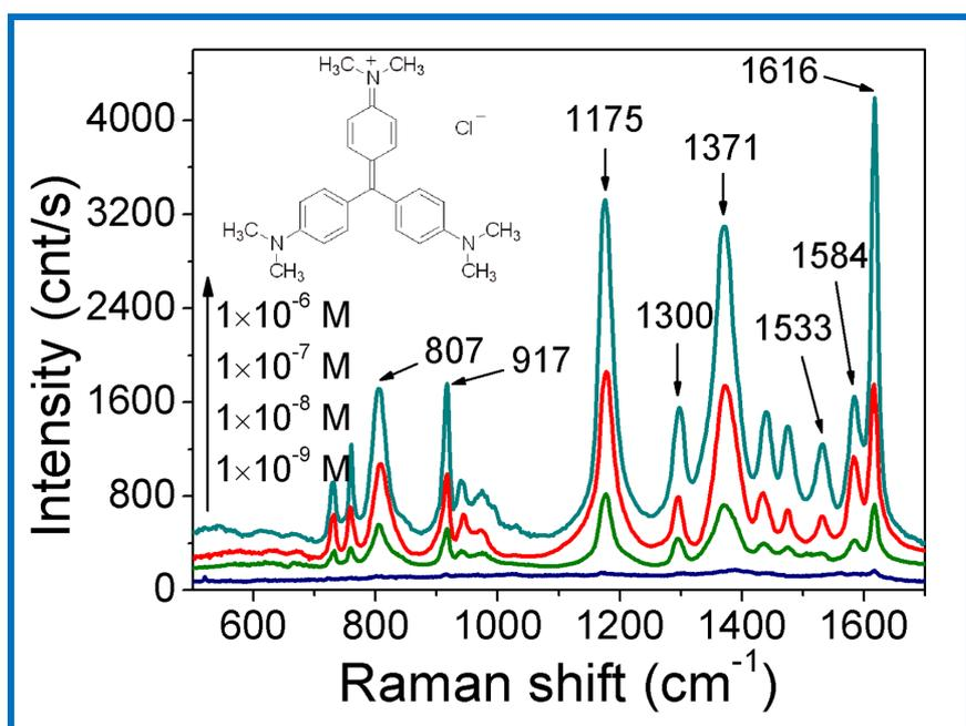
**Fig.S9** Series of SERS spectra of CV at different concentrations with NPGDF as SERS substrates. The primary vibrations of CV are confirmed according to the literatures.<sup>3,4</sup> The results clearly show that the determination capability of CV was below  $1 \times 10^{-8}$  M. That is, it verified further the high sensitivity of the NPGDF as substrate.
