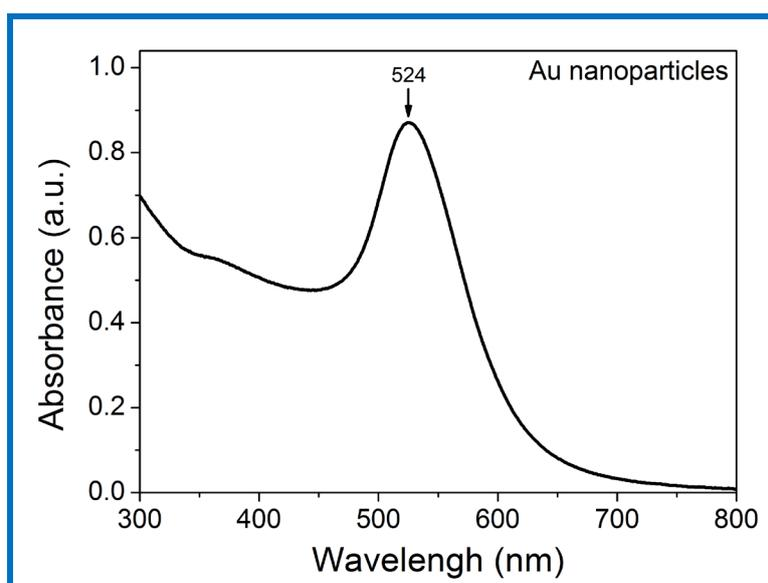
**Fig.S3** UV-vis absorption spectra of Au Nanoparticles (NPs). An obvious surface plasmonic absorption band is found around 524 nm. This symmetrical absorption band signifies the narrow size distribution of Au NPs.
