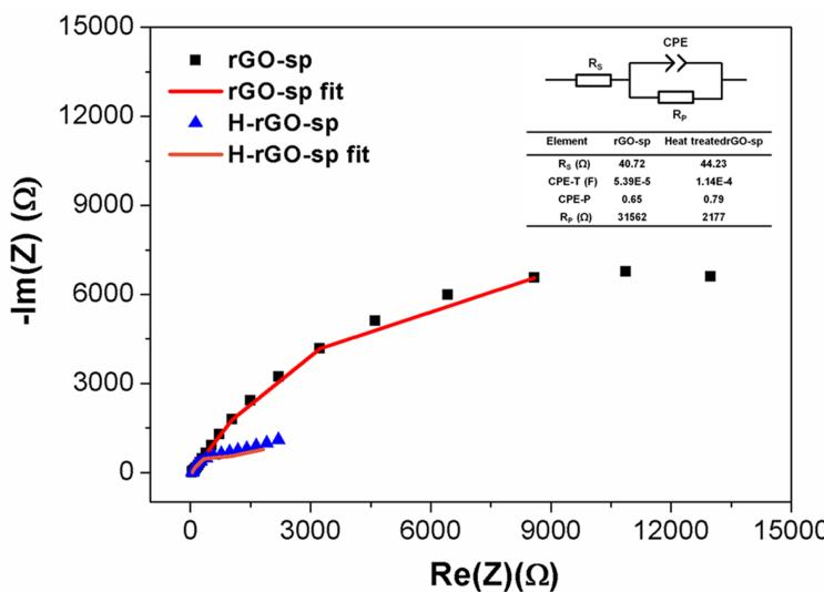
**Fig. S5** Impedance spectra of rGO-sp (black dot), H-rGO-sp (blue dot) modified glassy carbon electrodes in 5.0 mM  $\text{Fe}(\text{CN})_6^{3-/\text{4}-}$  containing 0.5 M KCl at 25 °C. Inset is the
