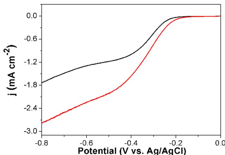
**Fig. S6** Linear sweep voltammetry curves for oxygen reduction on graphene (black line), H-rGO-sp (red line) modified GCE in  $\text{O}_2$ -saturated 0.1 M KOH solution (scan rate: 5  $\text{mV s}^{-1}$ , rotation rate: 1600 rpm).
