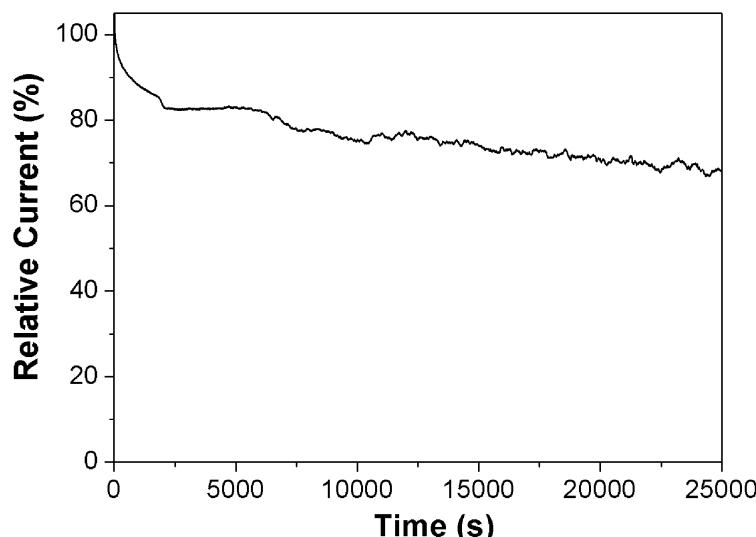
**Fig. S7** Current-time (*i-t*) chronoamperometric response of rGO modified GC electrode at -0.4 V in O<sub>2</sub> saturated 0.1 M KOH at rotation rate of 1600 rpm.
