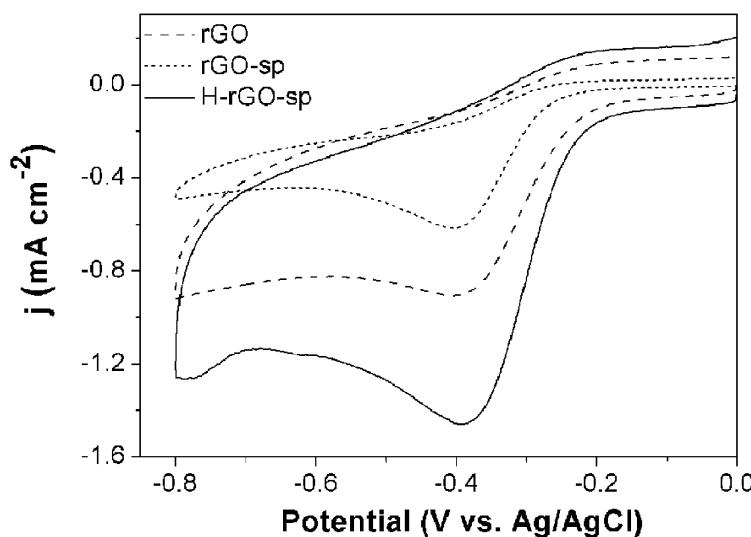
**Fig. S4** Cyclic voltammograms of Glassy carbon electrodes modified with rGO, rGO-sp and H-rGO-sp in 0.1 M KOH solution saturated with  $\text{O}_2$ . Scan rate, 100 mV/s.
