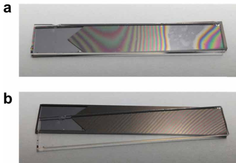
Figure S4. A control experiment without external voltage under identical temperature conditions. Graphene was transferred to SiO 2 over the entire area of the substrate and then these samples were bonded to glass substrates. Newton's rings are observed over the entire area of graphene (a),(b), which means that this area is not bonded. (b) Moreover, these samples are easily detached from each other.
