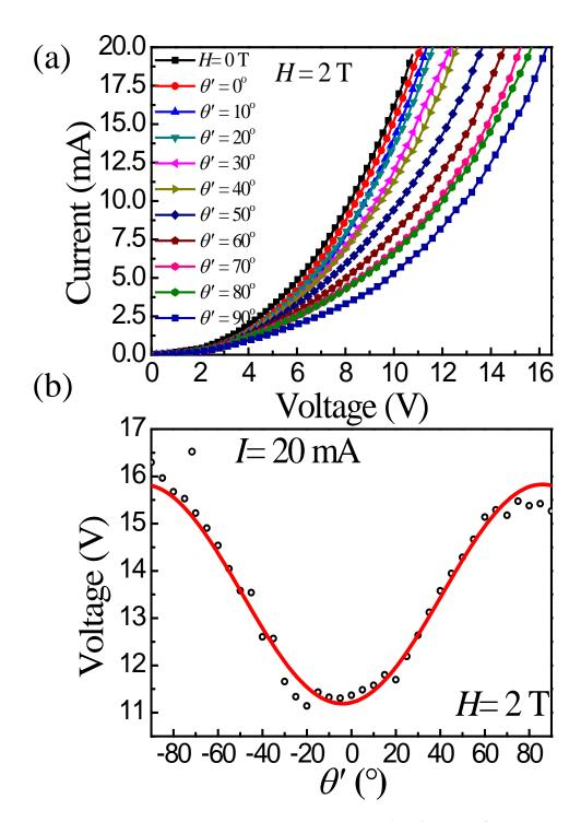
S. 1(a) shows the *I-V* characteristics of the *p-n* junction device for various magnetic field orientation in the x-z plane at room temperature. (b) shows the corresponding anisotropic MR curves at specified current I = 20 mA.
