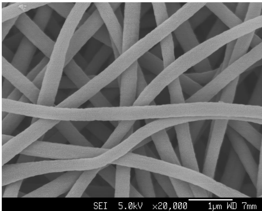
**Fig. S1.** FESEM image of carbonized electrospinning-derived carbon nanofibers, showing the nanofibrous morphology with uniform diameter and long length as well as the rough surface.
