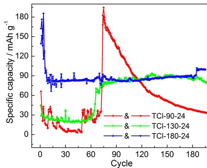
**Fig. S5.** The cycling capacity of the samples from 24 hrs' hydrothermal growth at 90 °C (TiO<sub>2</sub>-90-24), 130 °C (TiO<sub>2</sub>-130-24) and 180 °C (TiO<sub>2</sub>-180-24). The capacity shows severe instability along with the cycles.
