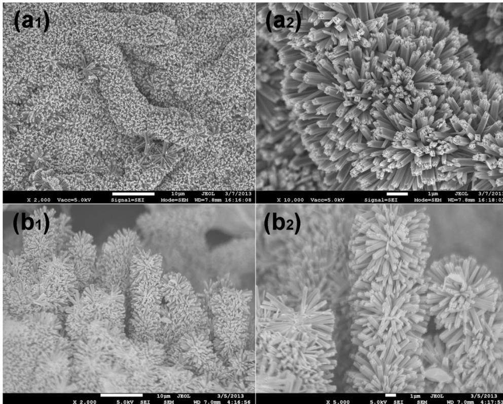
**Fig. S2.** The FESEM images of  $\text{TiO}_2$  nanostructures grown on carbon nanofibers using (a) titanium (IV) isopropoxide and (b) titanium (IV) butoxide as precursors, showing the morphology and dimension of  $\text{TiO}_2$  which is of separated nanorods with diameter of tens of nanometers.
