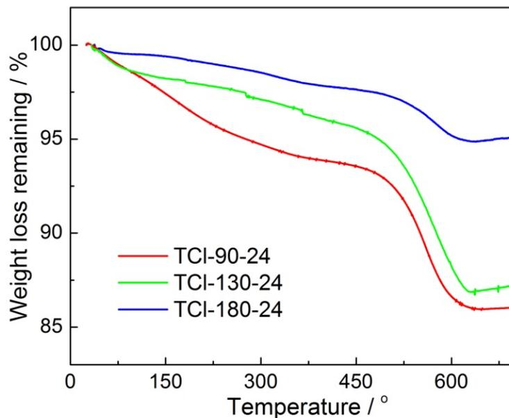
**Fig. S3.** TGA curves of the samples from 24 hrs' hydrothermal growth at 90 °C (TiO<sub>2</sub>-90-24), 130 °C (TiO<sub>2</sub>-130-24) and 180 °C (TiO<sub>2</sub>-180-24), showing that the content of TiO<sub>2</sub> is higher than 85 wt% in all samples.
