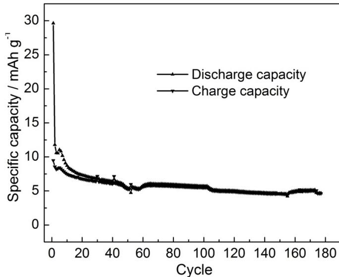
**Fig. S4.** The cycling capacity of pure carbon nanofibers (CNFs) at current rate of 50 mA g<sup>-1</sup> and voltage range of 1.0-2.8 V. It is shown that the capacity of CNFs is as low as about 5 mAh g<sup>-1</sup>, indicating the electrochemical inactivity of CNFs within the voltage range of 1.0-2.8 V.
