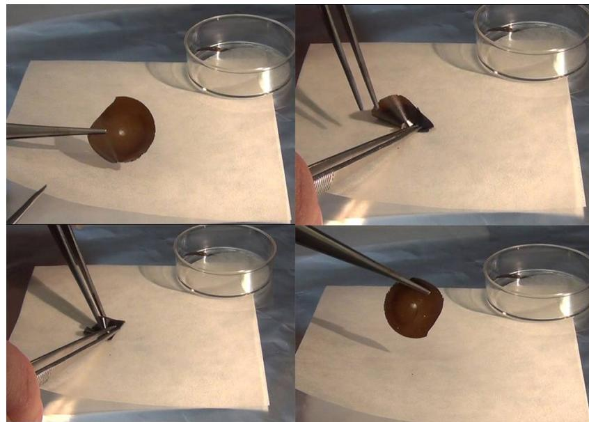
**Figure 1S** Folding of B-GO membrane does not result in breaking. H-GO membranes can be bent to certain extent but break on pieces when folded. See also video which shows B-GO and H-GO membranes folding difference.
