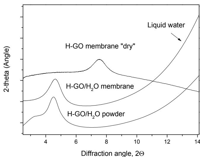
**Figure 4S.** Integrated XRD patterns of H-GO membrane in “dry” state (air exposed), H-GO membrane water immersed and reference sample of water immersed precursor H-GO powder. The background which starts above ~8 degrees is part of broad reflection from liquid water. Patterns recorded at 290K, radiation wavelength 0.99258 Å.
