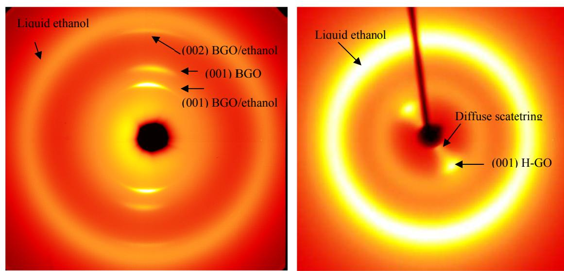
**Figure 6s** XRD images recorded for ethanol immersed samples of : a) B-GO membrane, no strong diffuse scattering is visible, only part of membrane is in solvated state,  $d(001)= d=9.05\text{\AA}$  and  $d(002)=4.52\text{\AA}$  for solvated phase,  $d(001)=6.95\text{\AA}$  for not solvated B-GO phase ; b) H-GO membrane, diffuse scattering similar to H-GO/water sample (Figure 5sa) is also observed.
