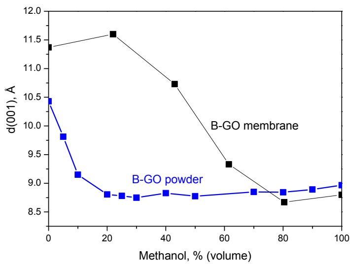
**Figure 8S.** Interlayer distance,  $d(001)$ , measured at 300K for GO in liquid water/methanol binary solvents: B-GO membrane ■ and B-GO powder ■.
