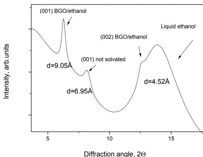
**Figure 7s.** Integrated patterns for XRD image of B-GO membrane immersed in liquid ethanol. Both solvated and not solvated phases identified in this sample, no change of relative intensity was observed for reflections form these phases with time. The data are interpreted as partial solvation of outer shell of the membrane while ethanol could not penetrate into inner core part of the membrane.
