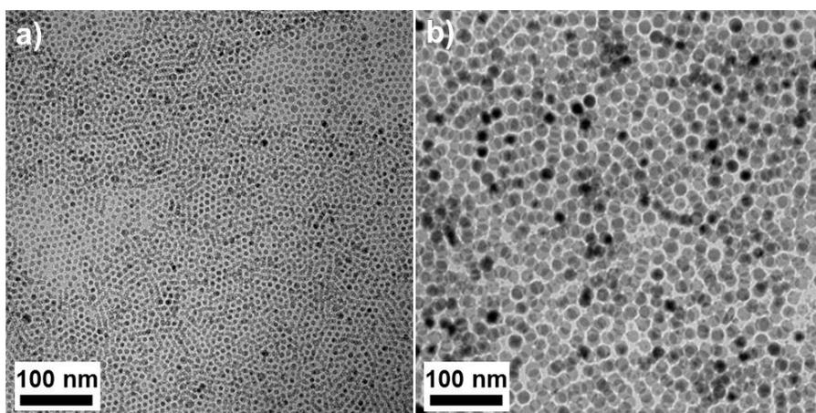
**Figure S5:** TEM images of superlattices formed by a) 7 nm and b) 17 nm spherical particles.
