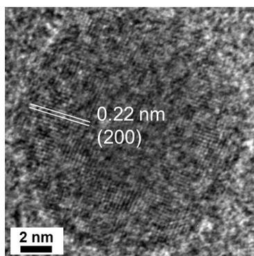
**Figure S4:** HRTEM image of 17 nm spherical particle. The lattice fringes are visible and have been indexed to MnO (200) reflections.
