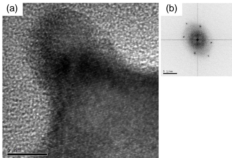
**Figure S7:** (a) A higher magnification TEM image of the corner of a typical octapod, clearly showing its single-crystal nature. The lattice fringe orientation is consistent with an underlying cubic structure with elongated [111] corners. (b) The associated Fourier transform.
