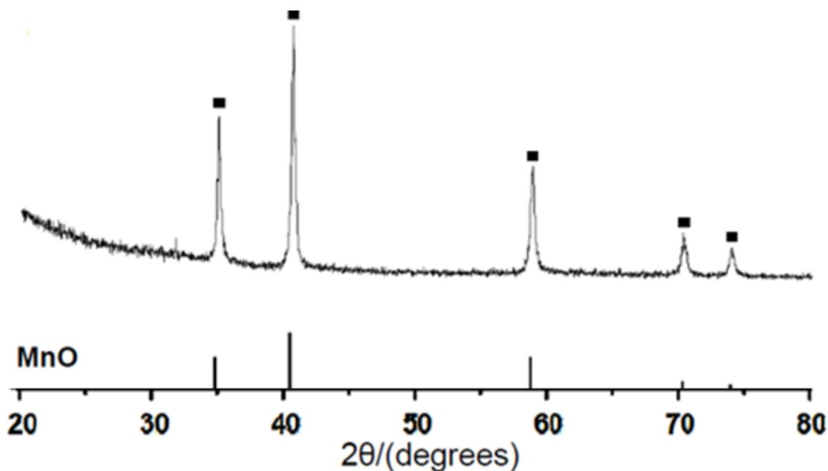
**Figure S2:** X-Ray Diffraction Pattern for as-obtained spherical MnO nanoparticles, showing agreement with cubic MnO reference pattern (JCPDS:07-0230).
