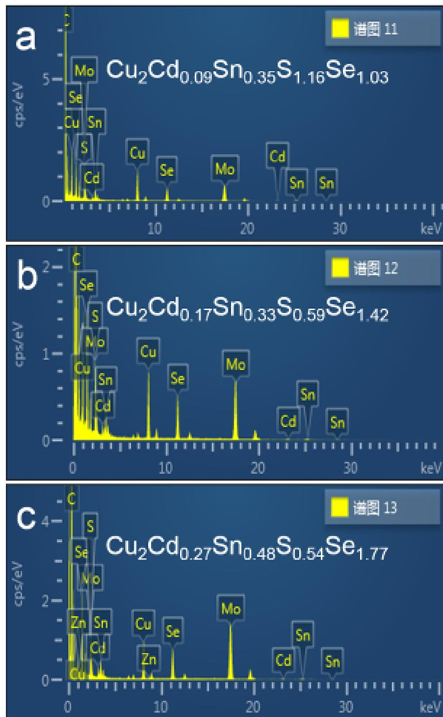
**Fig. S3** EDS spectra of nanocrystals prepared at different elevated reaction temperature. (a) 230 °C, (b) 250 °C, (c) 280 °C.
