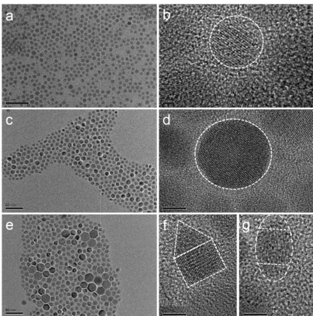
**Fig. S1** TEM and HRTEM images of nanocrystals prepared at different elevated reaction temperature. (a) and (b) 230 °C, (c) and (d) 250 °C, (e)-(g) 280 °C.
