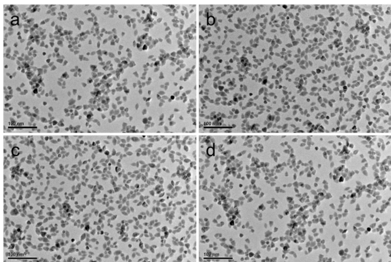
**Fig. S7** Low magnification TEM images of the polytypic CCTSSe nanocrystals for statistic calculation of the proportions of rugby-like and bullet-like nanocrystals: (a)  $\text{Cu}_2\text{Cd}_{0.59}\text{Sn}_{0.74}\text{S}_{0.26}\text{Se}_{2.45}$ , (b)  $\text{Cu}_2\text{Cd}_{0.79}\text{Sn}_{0.80}\text{S}_{0.75}\text{Se}_{2.70}$ , (c)  $\text{Cu}_2\text{CdSn}_{0.94}\text{S}_{0.41}\text{Se}_{3.07}$ , (d)  $\text{Cu}_2\text{Cd}_{1.13}\text{Sn}_{0.85}\text{S}_{0.60}\text{Se}_{3.11}$ .
