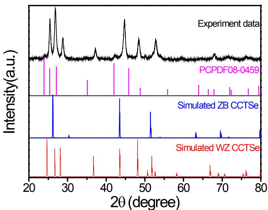
**Fig. S12** PXRD pattern of the polytypic CCTSSe nanocrystals synthesized with the Cu:Cd:Sn ratio in precursors kept as 2:1.6:1. For reference, the diffraction pattern of CdSe and the simulated diffraction patterns of WZ and ZB CCTSe are showed also.
