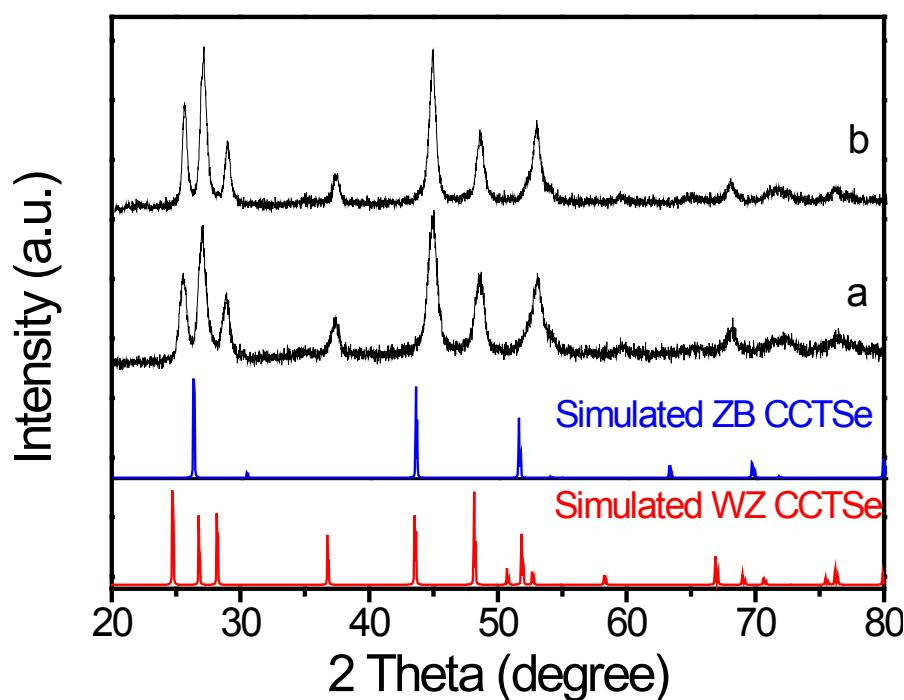
**Fig. S5** (a) and (b) PXRD patterns of the polytypic nanocrystals synthesized with 1 ml 1-DDT and 0.3 ml 1-DDT, respectively.
