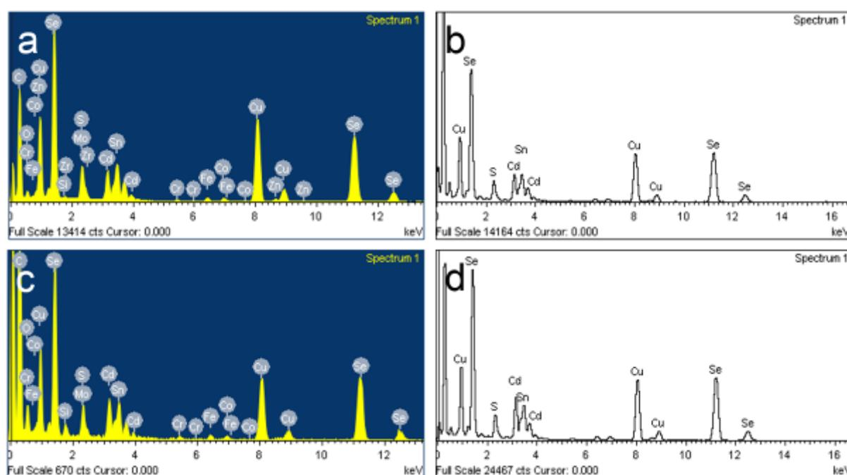
**Fig. S6** EDS spectra of the polytypic CCTSSe nanocrystals: (a)  $\text{Cu}_2\text{Cd}_{0.6}\text{Sn}_{0.7}\text{S}_{0.3}\text{Se}_{2.5}$ , (b)  $\text{Cu}_2\text{Cd}_{0.8}\text{Sn}_{0.8}\text{S}_{0.8}\text{Se}_{2.7}$ , (c)  $\text{Cu}_2\text{CdSn}_{0.9}\text{S}_{0.4}\text{Se}_{3.1}$ , (d)  $\text{Cu}_2\text{Cd}_{1.1}\text{Sn}_{0.9}\text{S}_{0.6}\text{Se}_{3.1}$ .
