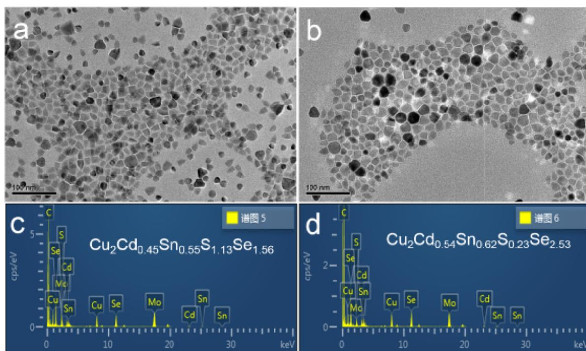
**Fig. S4** (a) and (b) TEM images of the polytypic nanocrystals synthesized with 1 ml 1-DDT and 0.3 ml 1-DDT, respectively. (c) and (d) EDS spectra of the polytypic nanocrystals synthesized with 1 ml 1-DDT and 0.3 ml 1-DDT, respectively.
