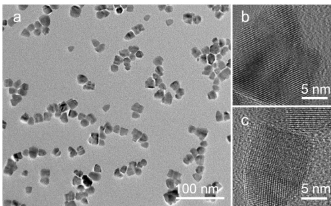
**Fig. S11** TEM and HRTEM images of the polytypic CCTSSe nanocrystals synthesized with the Cu:Cd:Sn ratio in precursors kept as 2:1.6:1.
