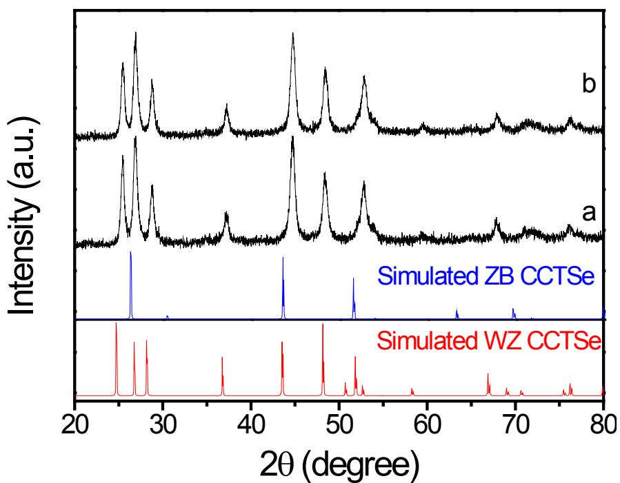
**Fig. S10** PXRD patterns of polytypic CCTSSe nanocrystals synthesized with different Cd source. (a) and (b) Cd(Ac)<sub>2</sub>, (c) and (d) CdO.
