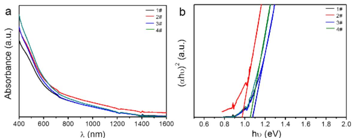
**Fig. S13** (a) UV-vis-NIR absorbance spectra of polytypic CCTSSe nanocrystals, (b)  $(\alpha h\nu)^2$  versus photon energy to low energy of polytypic CCTSSe nanocrystals.
