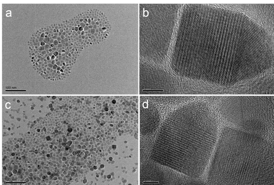
**Fig. S9** TEM and HRTEM images of the polytypic CCTSSe nanocrystals synthesized with different Cd source. (a) and (b) Cd(Ac)<sub>2</sub>, (c) and (d) CdO.
