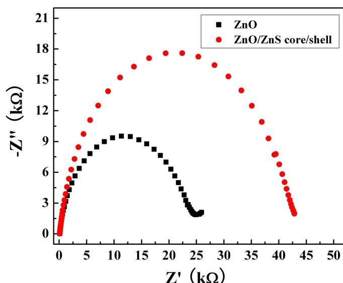
**Fig. S11** Electrochemical impedance spectroscopy of the ZnO-NRs and ZnO-NRs/ZnS nanoparticles electrodes, which were obtained in 0.5 M KCl solution containing 5.0 mM  $\text{Fe}(\text{CN})_6^{3-}/\text{Fe}(\text{CN})_6^{4-}$ .
