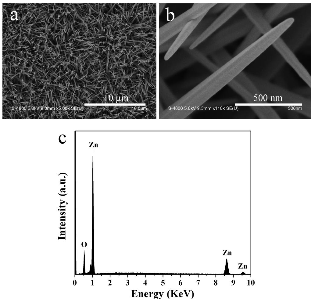
**Fig. S2** Morphology and structural characterization of the ZnO-NRs. (a, b) Low and high magnification FESEM images, respectively, and (c) EDX spectrum.
