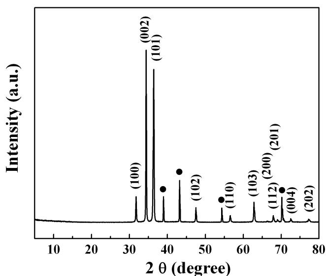
**Fig. S1** The XRD pattern of ZnO-NRs on the zinc substrate.
