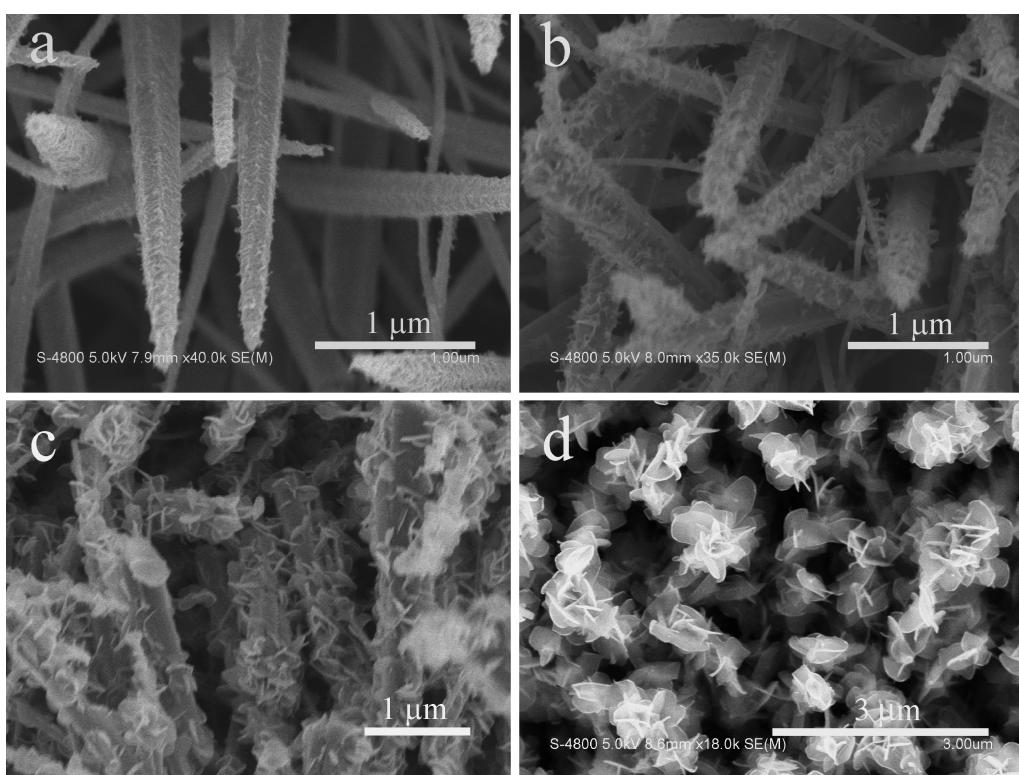
**Fig. S4** Typical FESEM images of the ZnO-NRs/ZnS·(HDA)<sub>0.5</sub>-NPs hierarchical heterostructure collected at different reaction times. (a) 10 min, (b) 30 min, (c) 60 min, and (d) 24 h.
