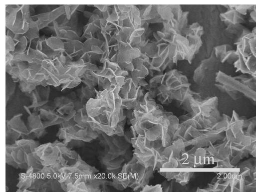
**Fig. S9** FESEM image of the ZnO-NRs/ZnS·(HDA)<sub>0.5</sub>-NPs product synthesized without the zinc substrate.
