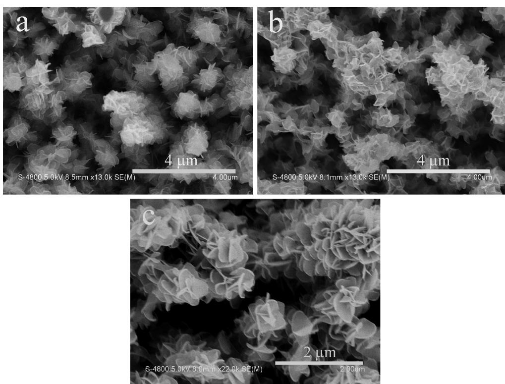
**Fig. S5** FESEM images of the ZnO-NRs/ZnS·(HDA)<sub>0.5</sub>-NPs hierarchical heterostructures synthesized under different concentrations of 1, 6-hexanediamin and Na<sub>2</sub>S. (a) The product with 4 mL of 1, 6-hexanediamine, (b) The product with 6 mL of 1, 6-hexanediamine, and (c) The product with Na<sub>2</sub>S concentration doubled.
