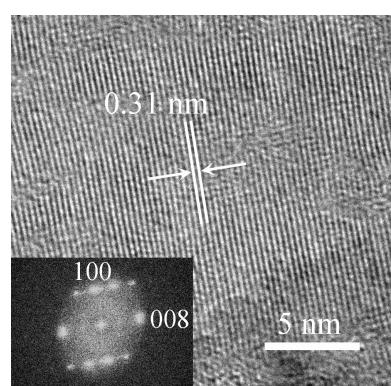
**Fig. S3** HRTEM image obtained at the edge of the nanoplate. The inset is the corresponding fast Fourier transform (FFT) spot diagram. The lattice spacings of 0.31 nm correspond to (008) lattice planes of hexagonal ZnS with 8H symmetry.
