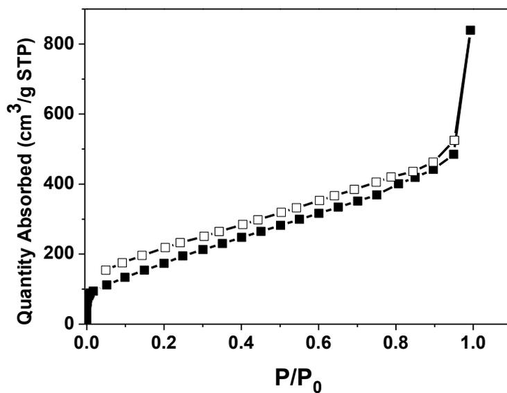
**Figure S10.** Nitrogen sorption isotherms for FTPA-HBCPN. Full symbols: adsorption, open symbols: desorption.
