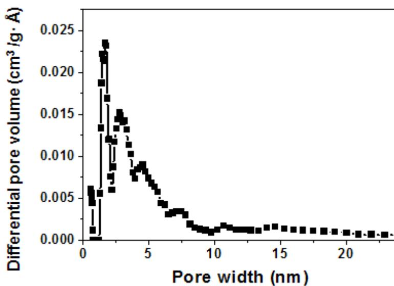
**Figure S11.** Pore size distributions for FTPA-CP calculated using NLDFT method (slit pore models, differential pore volume vs. pore width).
