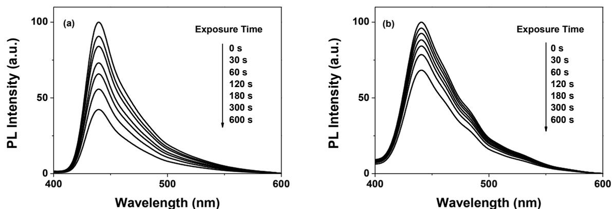
**Figure S13.** Fluorescence spectra of FTPA-HBCPN (a) and FTPA-LP (b) films upon exposure to TNT vapor.
