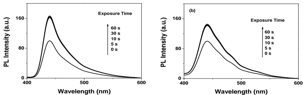
**Figure S16.** Fluorescence spectra of FTPA-HBCPN (a) and FTPA-LP (b) film upon exposure to toluene vapor.
