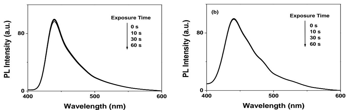
**Figure S17.** Fluorescence spectral changes of FTPA-HBCPN (a) and FTPA-LP (b) upon exposure to EtOH vapor.
