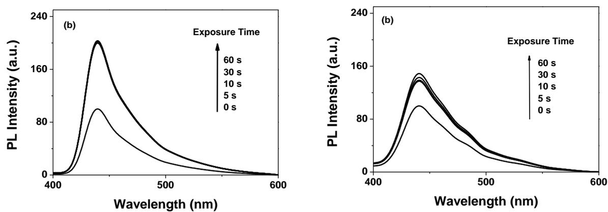
**Figure S18.** Fluorescence spectra of FTPA-HBCPN (a) and FTPA-LP (b) upon exposure to THF vapor.
