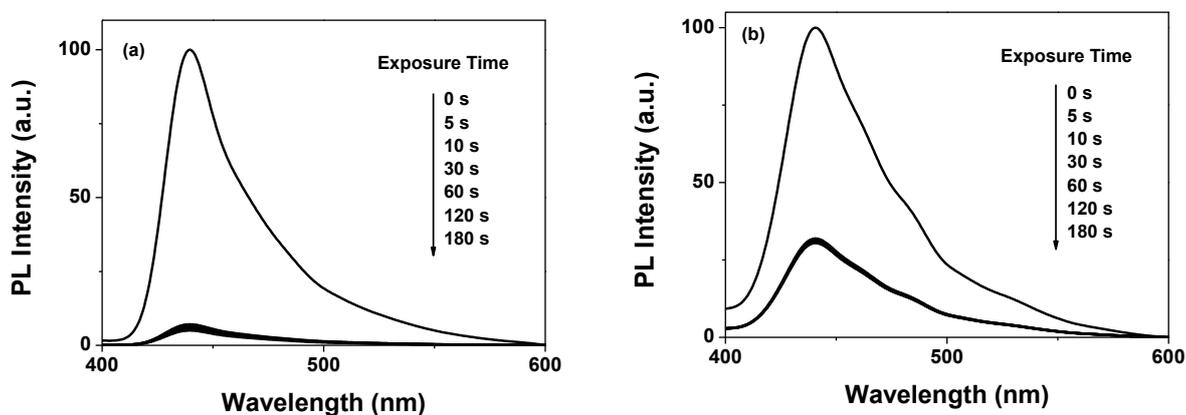
**Figure S15.** Fluorescence spectra of FTPA-HBCPN (a) and FTPA-LP (b) films upon exposure to NB vapor.
