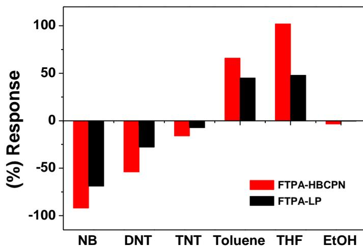
**Figure S19.** Changes in fluorescence emission intensity of spin-coated films upon exposure to the vapors of varied analytes at 60 s. A negative response indicates a quenching response in fluorescence intensity. A positive response indicates an enhancement response in fluorescence intensity.
