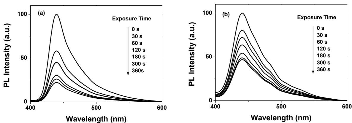
**Figure S14.** Fluorescence spectra of FTPA-HBCPN (a) and FTPA-LP (b) films upon exposure to DNT vapor.
