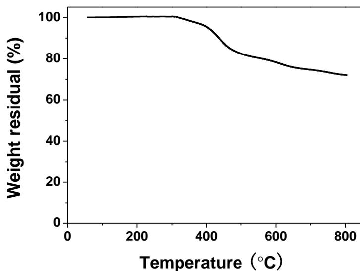
**Figure S3.** TGA curve recorded under N<sub>2</sub> for FTPA-HBCPN.
