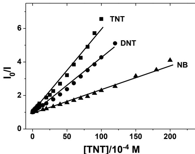
**Figure S12.** The Stern–Volmer plot of FTPA-HBCPN in THF solution against different nitroaromatics.
