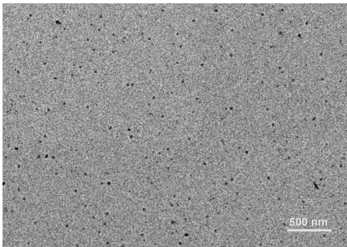
**Figure S5.** TEM image obtained by drop-casting a THF solution of FTPA-HBCPN onto a copper grid.
