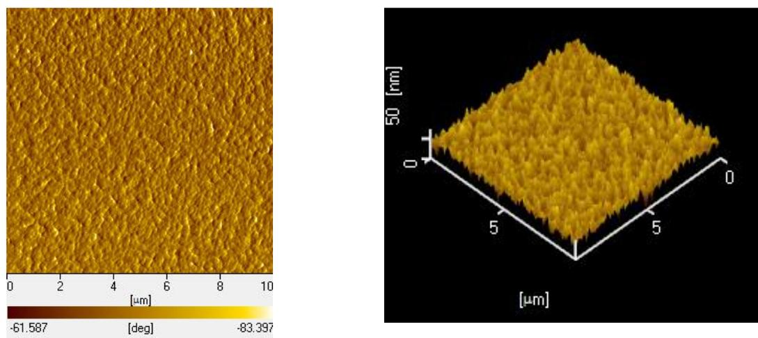
**Figure S8.** AFM phase and three-dimensional topography image of spin-casted thin film ( $10\ \mu\text{m}\times 10\ \mu\text{m}$ ) from the FTPA-HBCPN THF solution.
