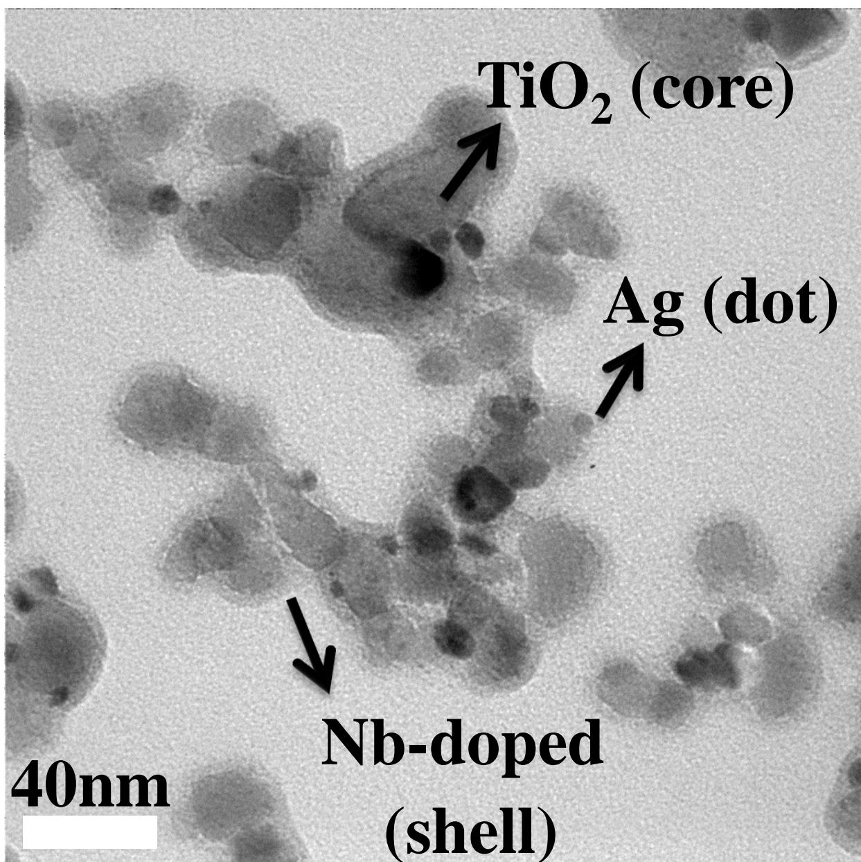
Fig. S1. Magnified EF-TEM micrograph of the bi-functional Nb-doped  $\text{TiO}_2/\text{Ag}$  ternary nanostructure.
