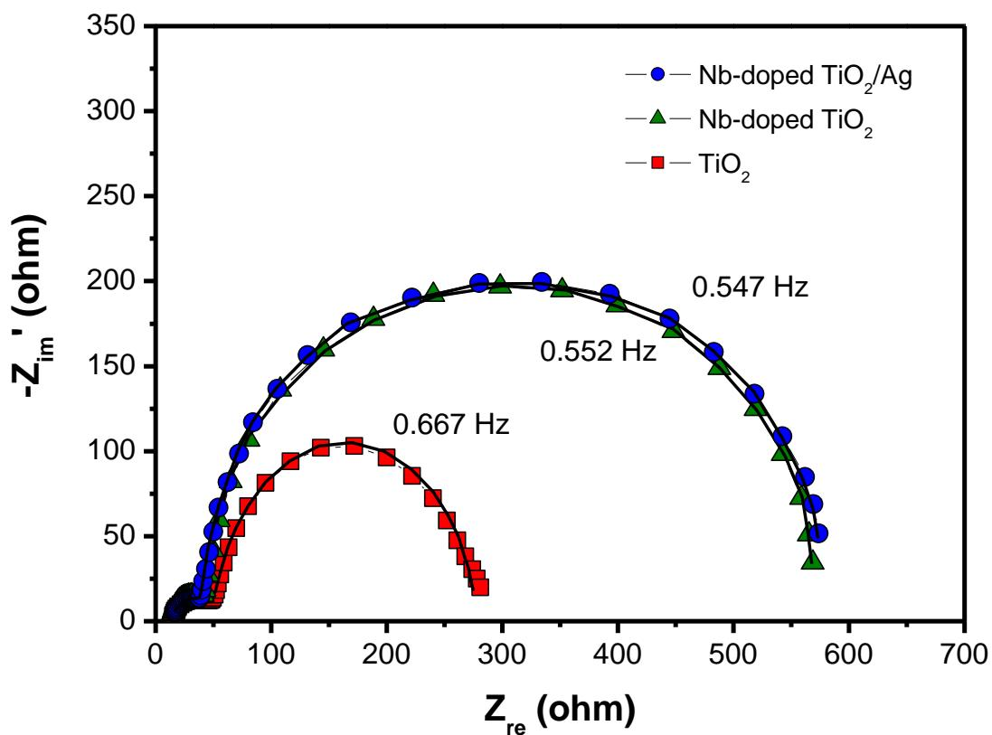
Fig. S3. EIS curves of DSSC with  $\text{TiO}_2$ , Nb-doped  $\text{TiO}_2$ , and Nb-doped  $\text{TiO}_2/\text{Ag}$  ternary nanostructure photoanode using a solid PEBII electrolyte measured at -0.65 V bias voltage under dark condition (100 kHz ~ 10 mHz). The fitting curves were obtained using Z-Plot software.
