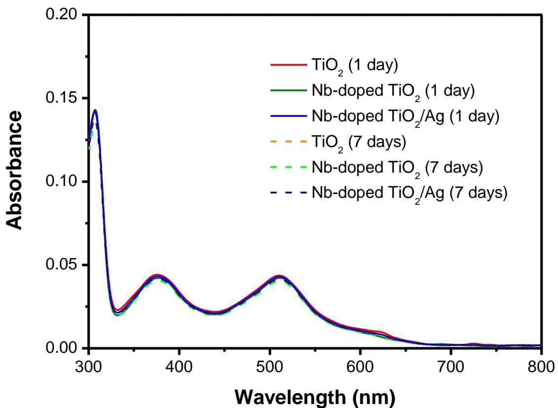
Fig. S2. UV-visible spectra of N719 dye loading on  $\text{TiO}_2$ , Nb-doped  $\text{TiO}_2$  and Nb-doped  $\text{TiO}_2/\text{Ag}$  ternary nanostructure after 1 and 7 days.
