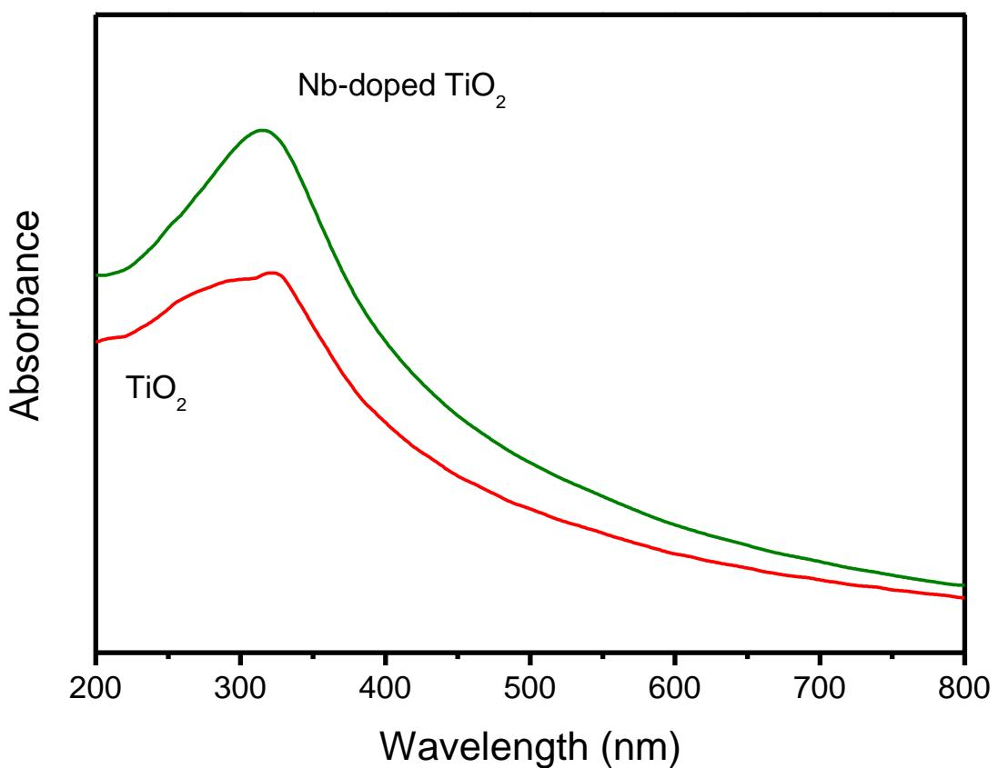
Fig. S4. Optical absorption spectra of the  $\text{TiO}_2$  and Nb-doped  $\text{TiO}_2$  photoanode.
