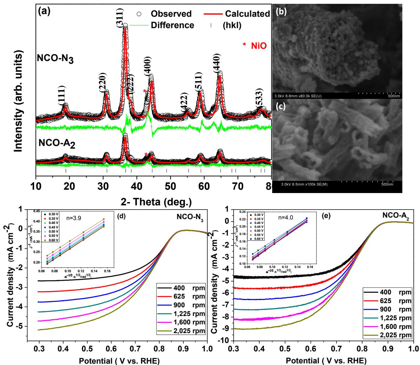
**Fig. S1** (a) Rietveld refined XRD pattern of NCO-N<sub>3</sub>, NCO-A<sub>2</sub>. The continuous line is fitted data and symbols are experimental data. The differences patterns and Miller indices (h k l) are shown, (b) SEM image of NCO-N<sub>3</sub>, (c) SEM image of NCO-A<sub>2</sub>. (d, e) Oxygen reduction polarization curves for NCO-N<sub>3</sub>, NCO-A<sub>2</sub> at different rotation rates with a scan rate of 5 mV/s. Inset shows the Koutecky–Levich plot at different potentials.
