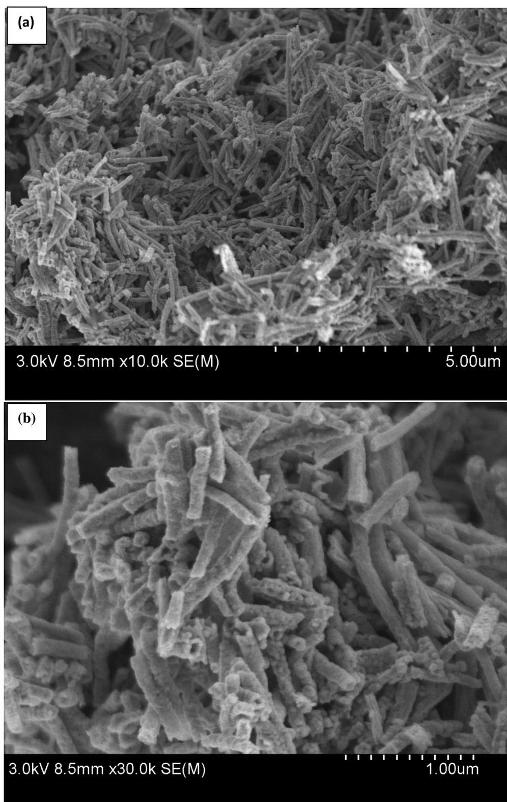
**Fig. S2** (a) Low and (b) high magnification SEM images of NCO-A<sub>1</sub> catalyst. The SEM image (b) clearly shows the porous tubular morphology of NCO-A<sub>1</sub> sample.
