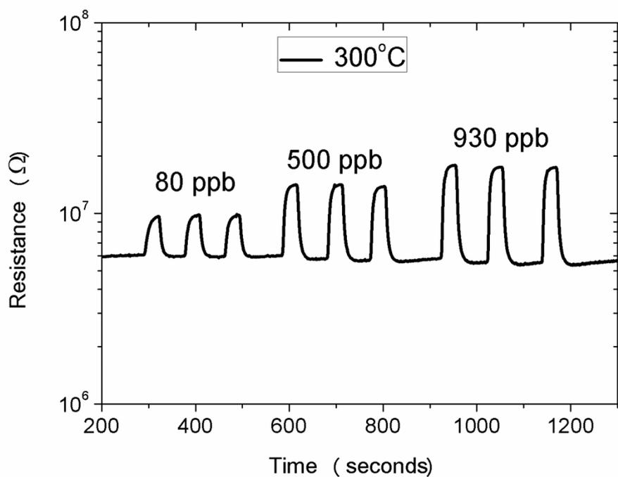
**Figure S2.** Ozone gas response of  $\alpha\text{-Ag}_2\text{WO}_4$  nanorods at 300°C exposure to different ozone concentrations.
