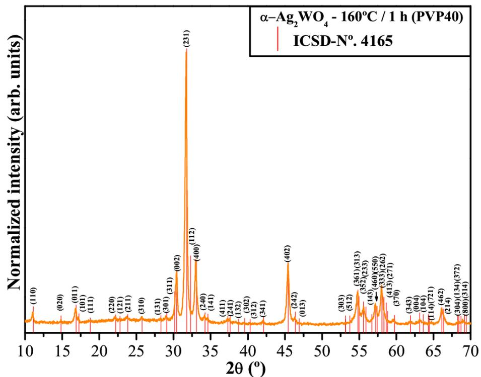
Figure 1S. X-ray diffraction pattern of  $\alpha\text{-Ag}_2\text{WO}_4$  powder obtained by MAH method.
