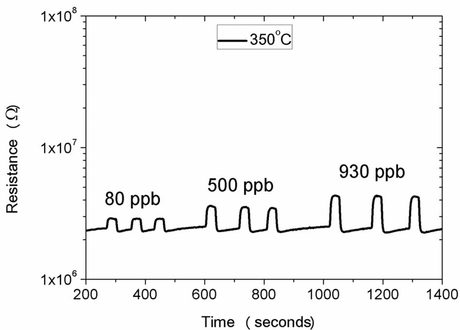
**Figure S3.** Ozone gas response of  $\alpha\text{-Ag}_2\text{WO}_4$  nanorods at 350°C exposure to different ozone concentrations.
