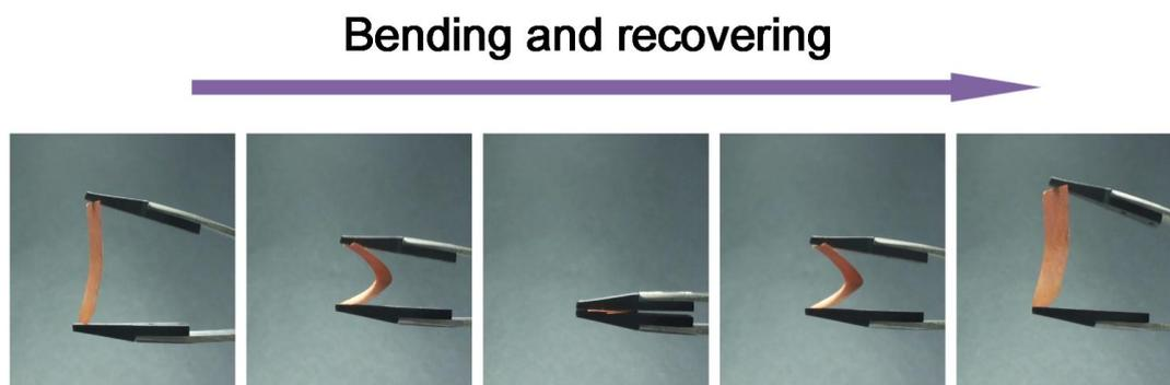
**Fig. S5** Optical images presenting the promising flexibility of  $\gamma\text{-Fe}_2\text{O}_3\text{@SNF}$  membranes by facilely bending and recovering.
