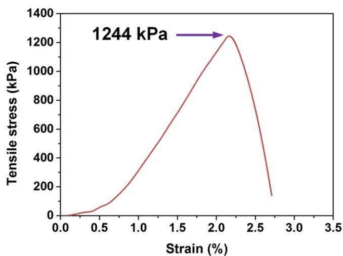
**Fig. S6** Stress-strain curve of  $\gamma\text{-Fe}_2\text{O}_3\text{@SNF}$  shows the robust strength of 1244 kPa.
