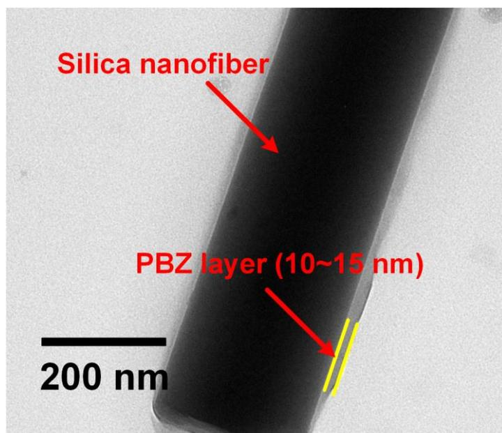
**Fig. S3** TEM image of the PBZ/SNF membranes shows the well coated PBZ layer with the uniform thickness of 10~15 nm.
