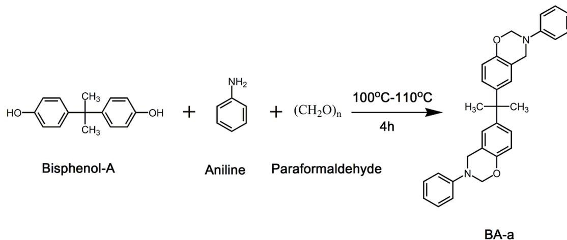
**Fig. S1** Schematic representation of the synthesis of BA-a via Mannich reaction.
