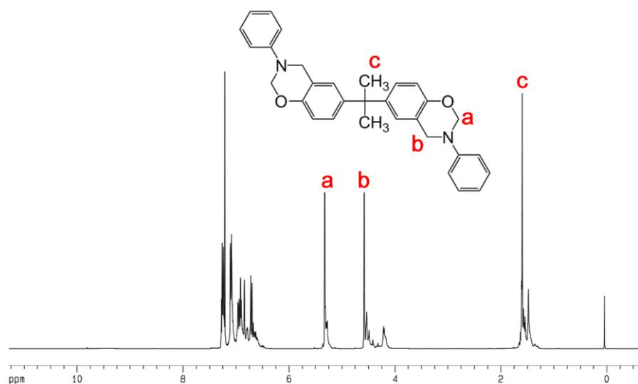
**Fig. S2**  $^1\text{H}$  NMR spectrum of as-synthesized BA-a,  $d\text{-CHCl}_3$  was used as the solvent.
