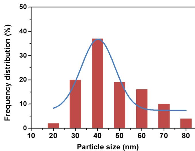
**Fig. S4** Histogram showing the size distribution of  $\gamma$ -Fe<sub>2</sub>O<sub>3</sub> nanoparticles.
