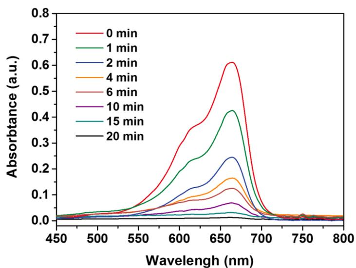
**Fig. S7** UV-Vis spectra of MB solution ( $1 \times 10^{-5}$  M) and after treatment with  $\gamma\text{-Fe}_2\text{O}_3\text{@SNF}$  for various time.
