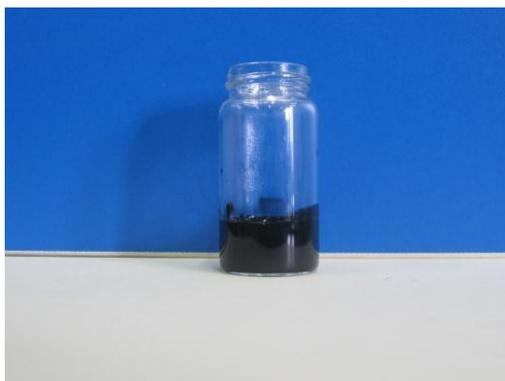
**Fig. S4** Photograph of the cellulose nanofibers/single-walled carbon nanotubes suspension
