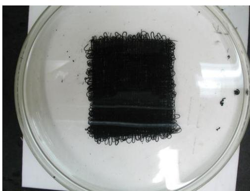
**Fig. S5** Photograph of the cellulose nanofibers/single-walled carbon nanotubes hybrid non-woven macrofiber mat in ethanol coagulation bath
