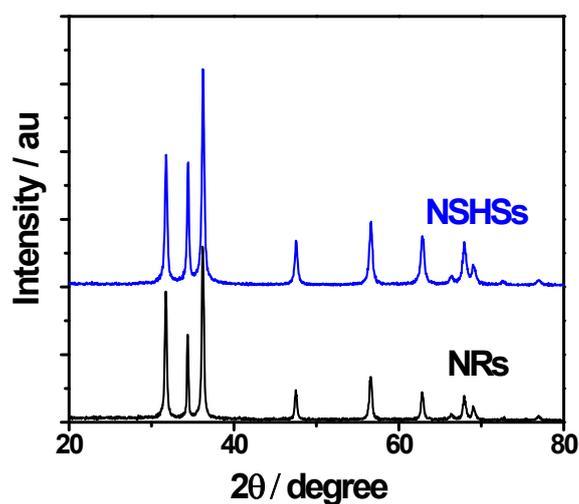
**Figure S1.** X-ray diffraction (XRD) patterns of the nanorods (NRs) and nanosheets-based hierarchical structures (NSHSs).
