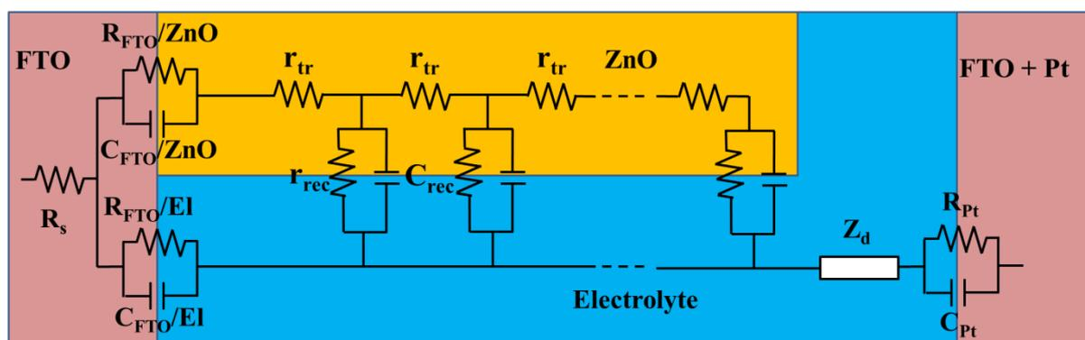
**Figure S5.** The transmission line model of DSCs, where the orange and blue parts represent the two channels of ZnO and electrolyte, respectively.  $r_{tr}$  represents the electron transport resistance in ZnO film;  $r_{rec}$  is the charge-transfer resistance between electrons in the ZnO film and  $I_3^-$  in the electrolyte,  $C_{rec}$  is the
