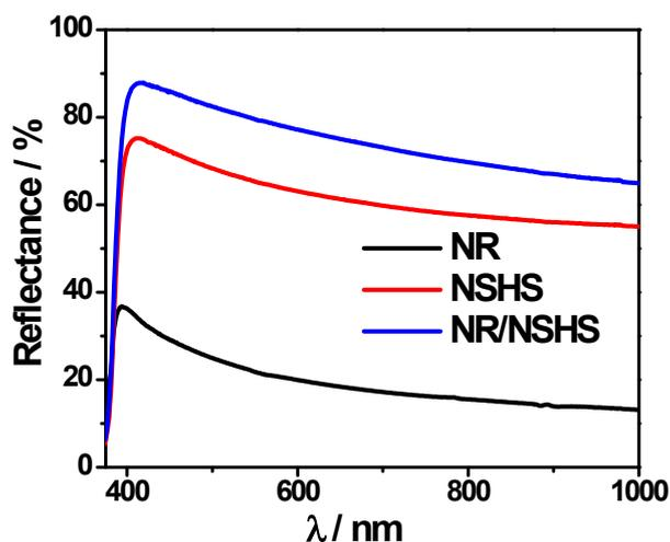
**Figure S3.** Reflectance spectra of the NR, NSHS, and the composite NR/NSHS photoanodes used for DSCs fabrications in this work
