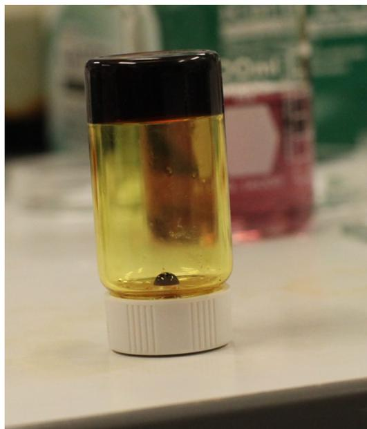
**Figure S2.** PEO-based polymer gel electrolyte at 100 °C, highly viscous.
