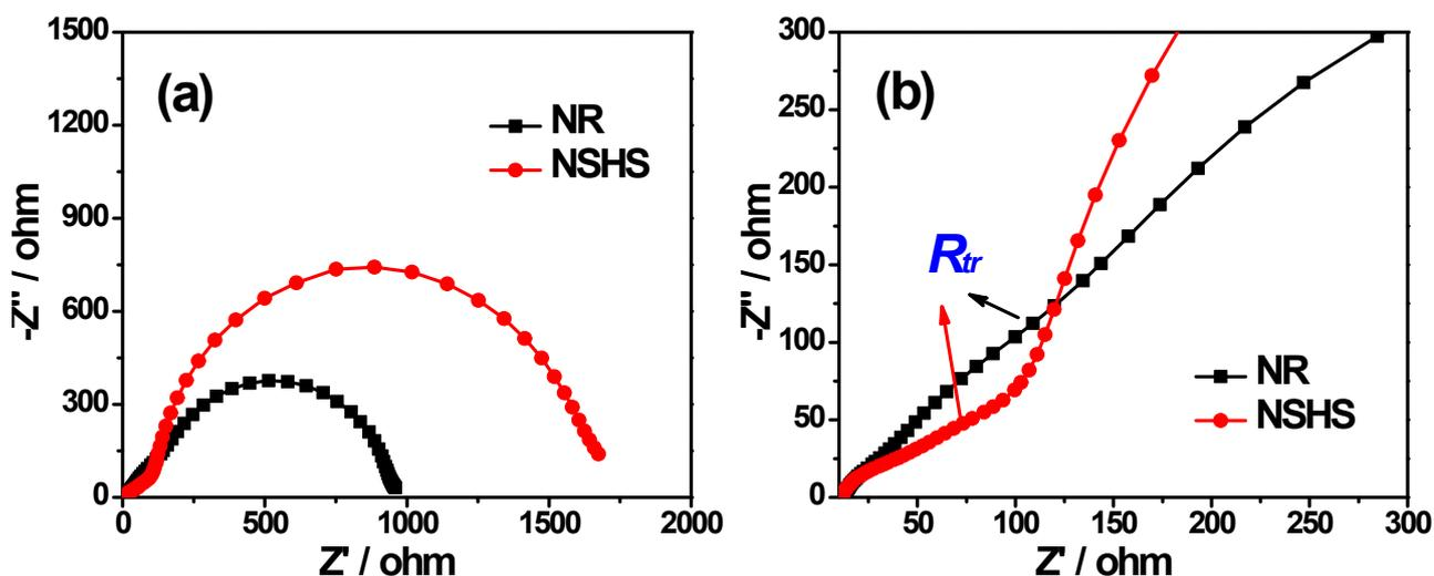
**Figure S6.** (a) Nyquist plots of the quasi-solid DSCs based on NR and NSHS under a bias of -0.56V, thicknesses of these two films were  $\sim 15 \mu\text{m}$ ; (b) the enlarged parts of the high frequency region. According to the transmission line model and above EIS analysis, electron transport resistance ( $R_{tr}$ ) within the NSHS photoanode was obviously smaller than that within NR.
