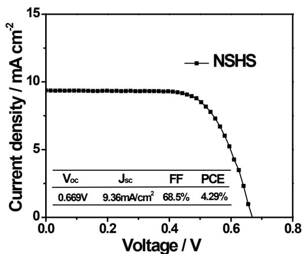
**Figure S4.**  $J$ - $V$  curves of the quasi-solid DSCs based NSHS, film thick was  $\sim 39.2 \mu\text{m}$
