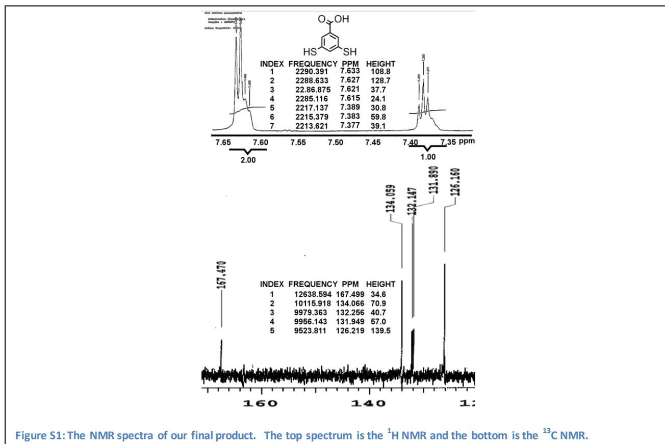
Figure S1: The NMR spectra of our final product. The top spectrum is the <sup>1</sup>H NMR and the bottom is the <sup>13</sup>C NMR.
