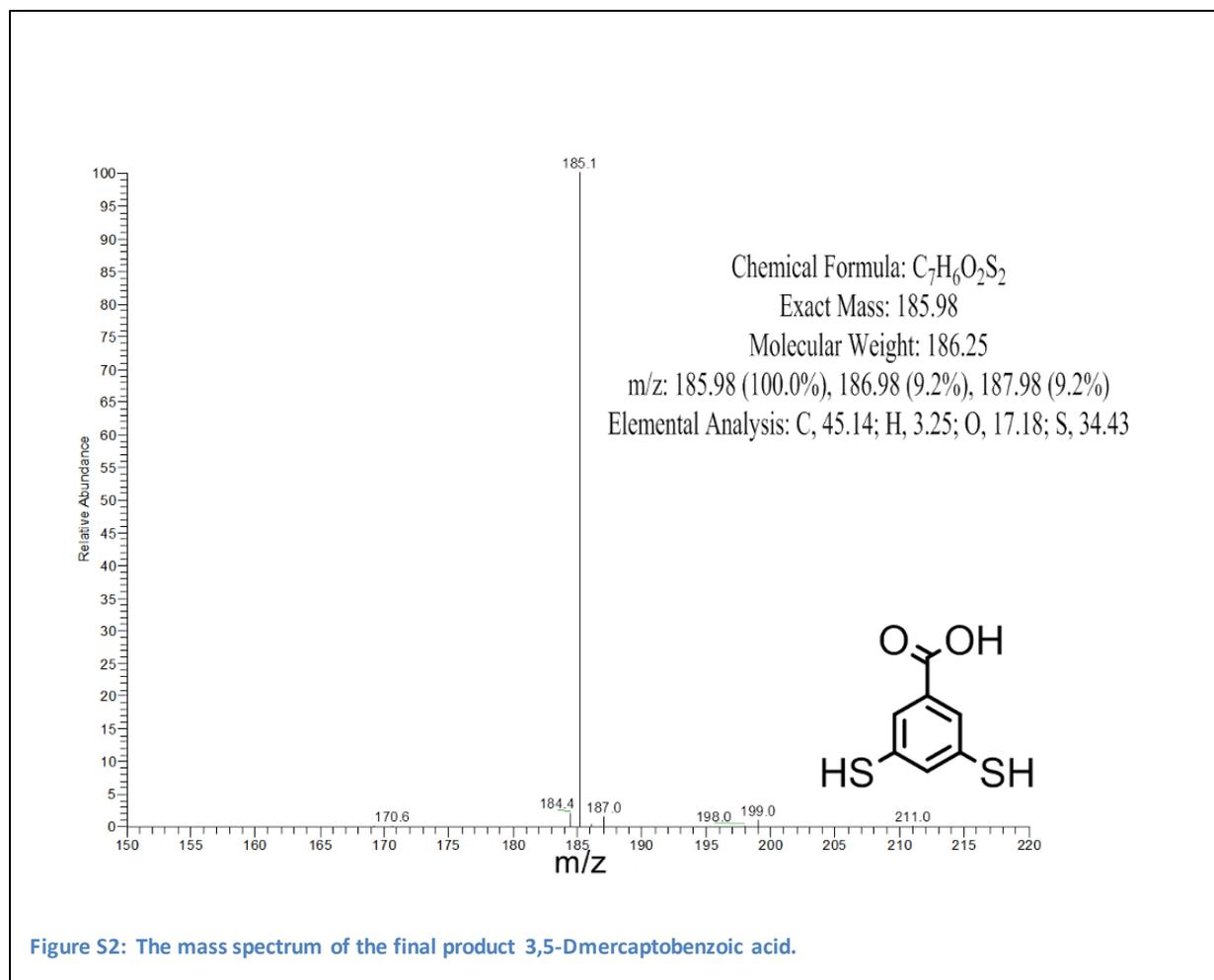
Figure S2: The mass spectrum of the final product 3,5-Dmercaptobenzoic acid.
