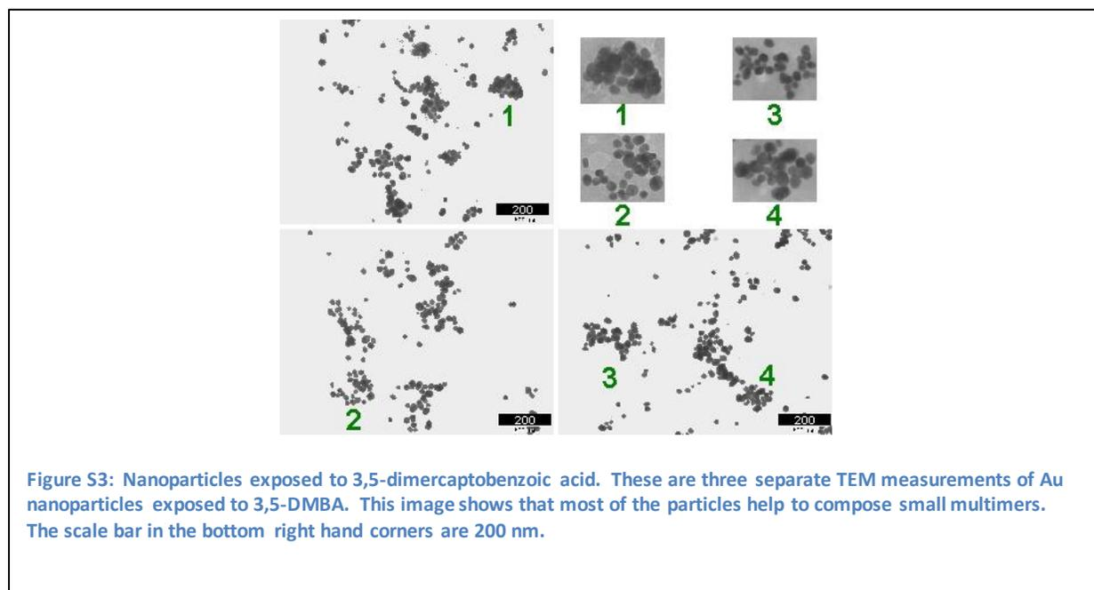
Figure S3: Nanoparticles exposed to 3,5-dimercaptobenzoic acid. These are three separate TEM measurements of Au nanoparticles exposed to 3,5-DMBA. This image shows that most of the particles help to compose small multimers. The scale bar in the bottom right hand corners are 200 nm.
