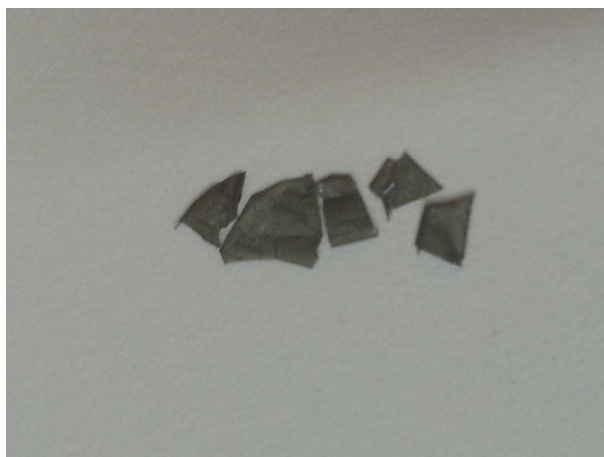
Fig. S7 The photograph of the Ag-nanosheet-grafted PA-nanofiber membrane which is tailored into several pieces with any desired shape.
