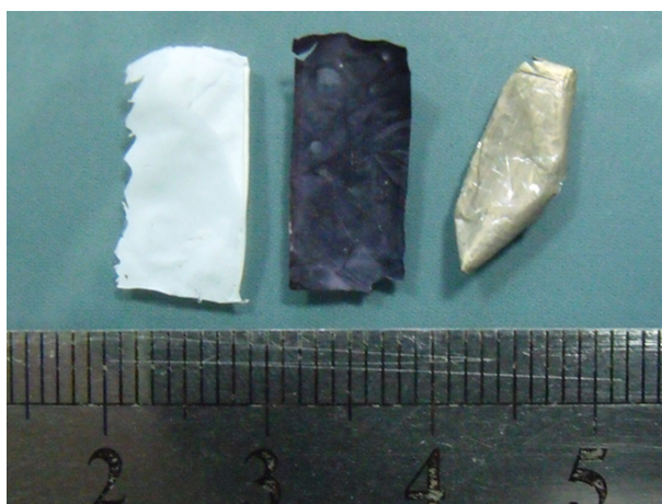
Fig. S2 The photographs of bare PA-nanofiber membrane, Au-nanoparticle-grafted PA-nanofiber membrane and Ag-nanosheet-grafted PA-nanofiber membrane from left to right, respectively.
