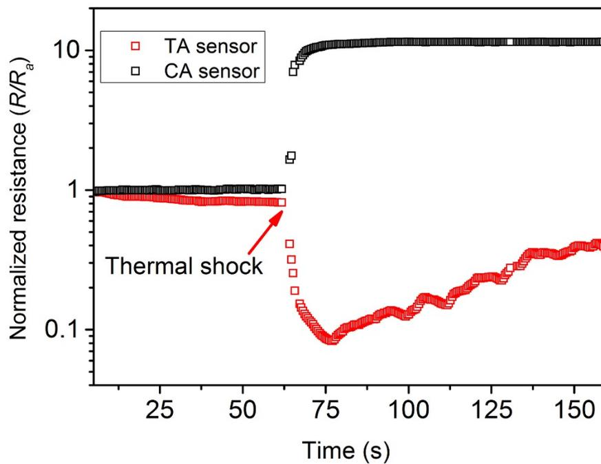
Fig. S5 The resistance change of the TA and CA sensor under a thermal shock (rapid heating from room temperature to 80°C). The slight decrease in the resistance of the TA sensor in the first minute is most probably caused by the self-heating effect.<sup>2</sup>
