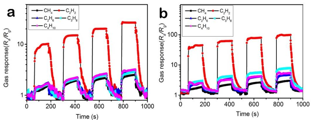
Fig. S7 Transient responses of the TA sensors made from ZnO (a) and SnO<sub>2</sub> (b) to different hydrocarbon gases.
