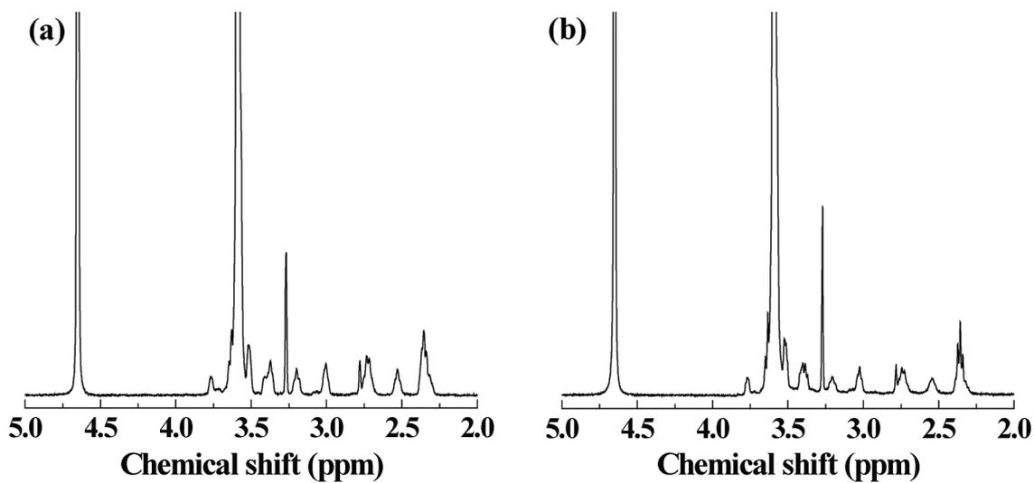
**Figure S1.** <sup>1</sup>H NMR spectra of the G2-*m*PEG dendrimers (a) and PEGylated Au DENPs (b).
