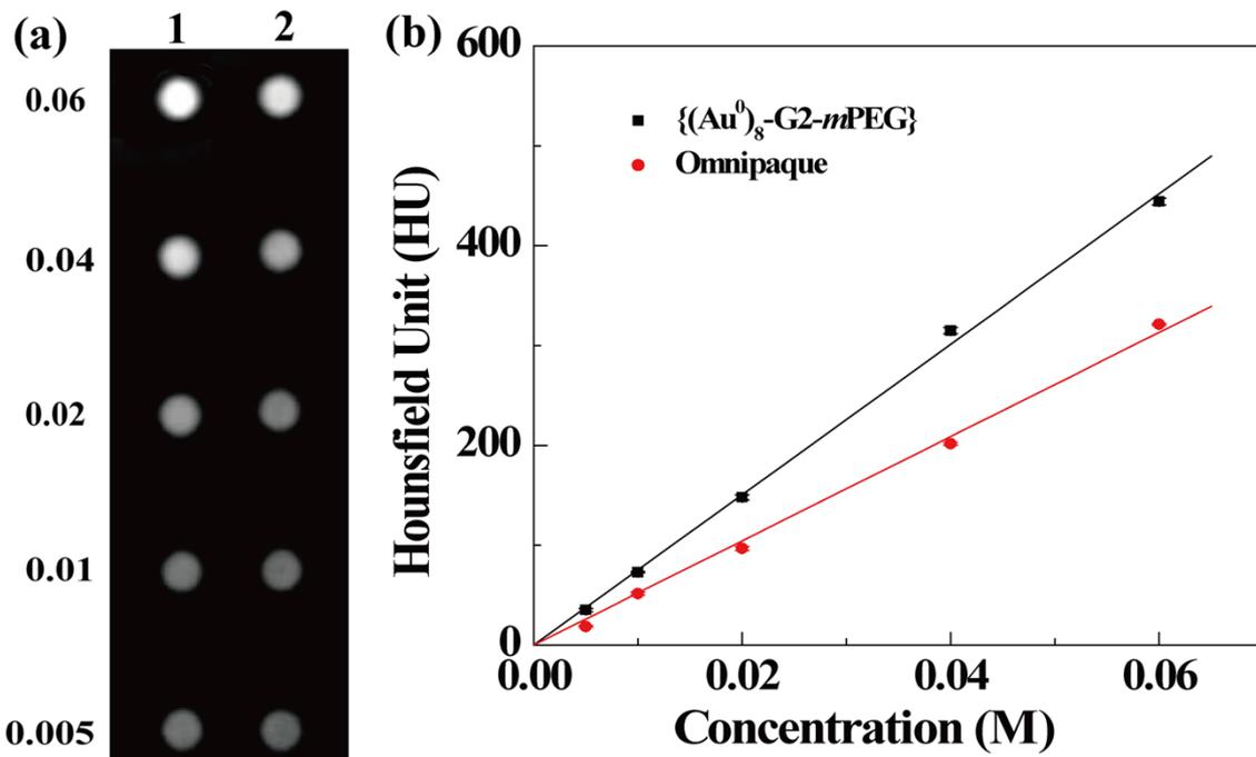
**Figure S7.** (a) CT images of (1) PEGylated Au DENPs and (2) Omnipaque with different concentrations. (b) X-ray attenuation intensity (HU) of PEGylated Au DENPs and Omnipaque as a function of the molar concentration of active element (Au or iodine).
