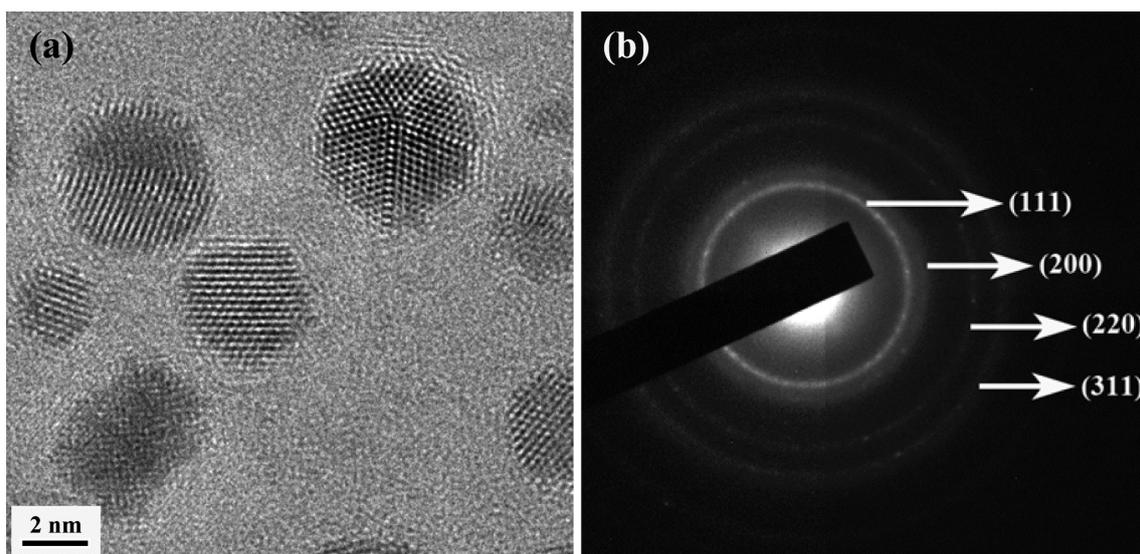
**Figure S3.** A typical high-resolution TEM image (a) and SAED pattern (b) of PEGylated Au DENPs.
