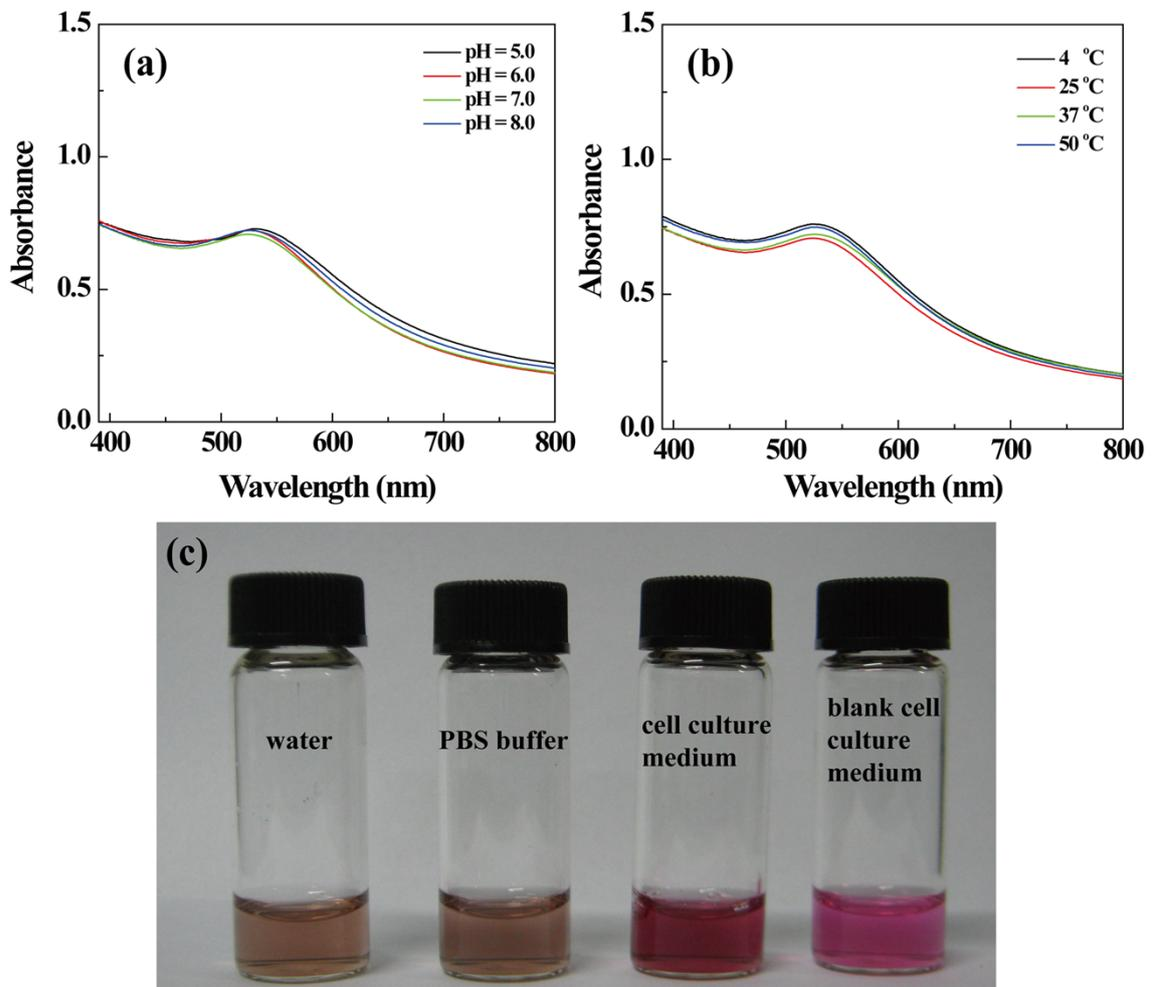
**Figure S4.** UV-Vis spectra of PEGylated Au DENPs under different pH (a) and temperature (b) conditions. The photographs of the as-prepared PEGylated Au DENPs dispersed in different media and the blank cell culture medium are shown in (c).
