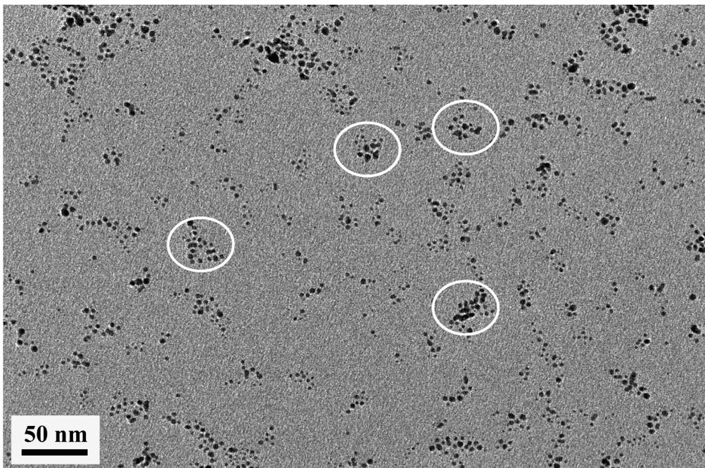
**Figure S2.** A large scale TEM image of the synthesized PEGylated Au DENPs.
