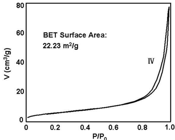
**Fig. S4.** N<sub>2</sub> adsorption-desorption isotherm curve of the *p* Fe<sub>3</sub>O<sub>4</sub> nanoparticles.
