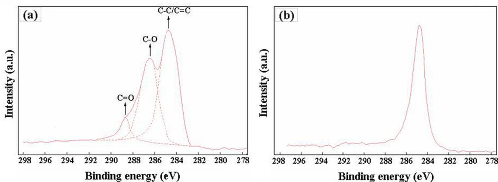
**Fig. S1.** The  $C_{1s}$  XPS spectra of GO and GN.
