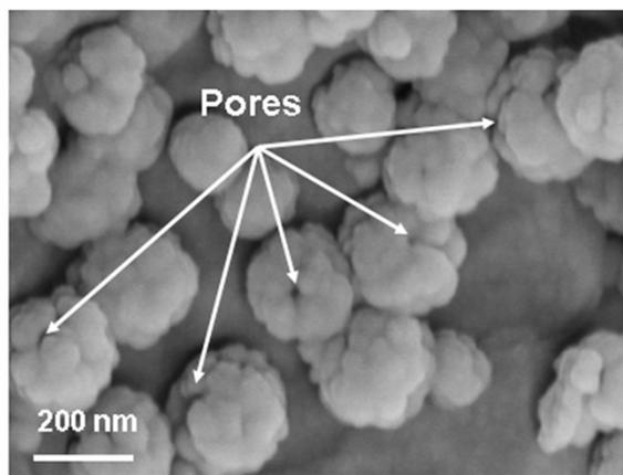
**Fig. S2.** FE-SEM image of the  $p\text{Fe}_3\text{O}_4$  nanoparticles.
