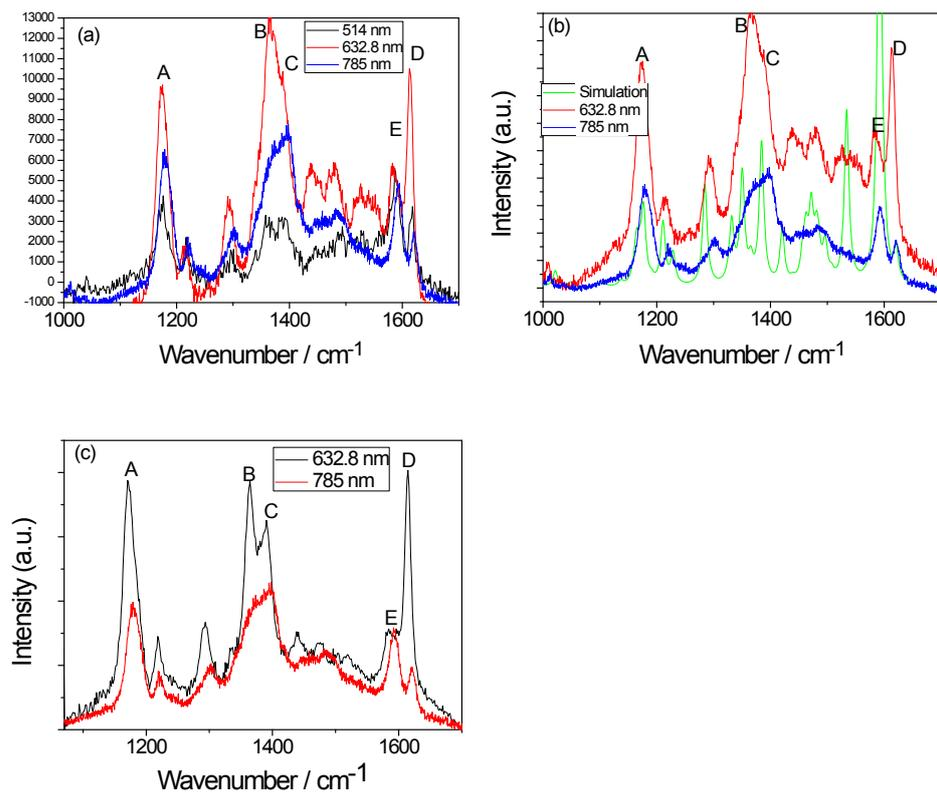
Figure S1. (a) The SERS spectra of MG in Ag sol excited at different frequencies, and (b) the comparison between the simulated normal Raman spectrum and experimental SERS spectra, where the simulated normal Raman frequencies were scaled by 0.965, and (c) the comparison between TERRS excited at 632.8 nm and SERS excited at 785 nm.
