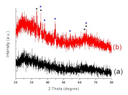
**Figure SI 1.** XRD results for alumina template (a) and  $Fe_2O_3$ - $Fe_3O_4$  mixture nanostructures obtained after heat treatment at 325 °C in flowing  $H_2$  gas (b). Black and blue asterisks indicate  $\alpha$ - $Fe_2O_3$  and  $Fe_3O_4$  structures, respectively.
