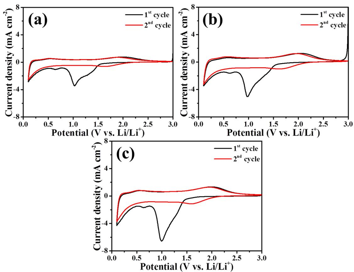
**Fig. S4** Cyclic voltammograms of (a) ST-450, (b) ST-500 and (c) ST-600 recorded by a scan rate of 1.0 mV s<sup>-1</sup> between 0.1 V and 3.0 V in 1 M LiPF<sub>6</sub> EC/DEC (1:1 w/w) solution.
