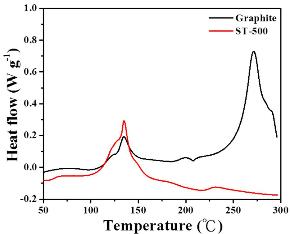
**Fig. S5** DSC thermograms of lithiated electrodes obtained in N<sub>2</sub> atmosphere with the heating rate of 10 °C min<sup>-1</sup>.
