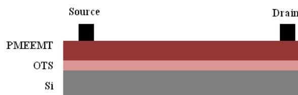
**Fig. S2** Schematic representation of metal-insulator-semiconductor (MIS) device structure.
