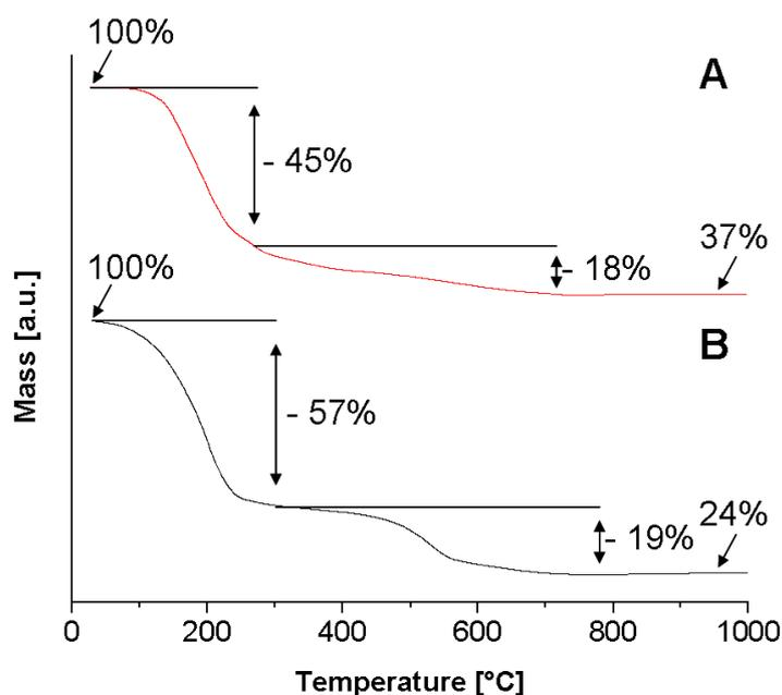
**Figure S7.** Comparison of the thermo gravimetric measurements under nitrogen atmosphere A) in the absence and B) in the presence of ammonium chloride. A different dependency of the mass lost on the temperature is observed. The presence of ammonium chloride leads to an
