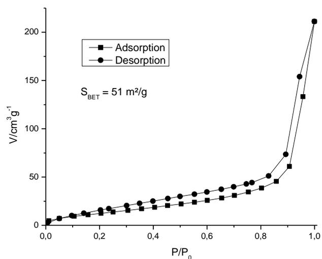
**Figure S3.** In order to determine the surface area of the Zn<sub>1.7</sub>GeN<sub>1.8</sub>O particles synthesized in the presence of ammonium chloride at 800 °C, a Brunauer-Emmett-Teller (BET) –slope using nitrogen gas was measured. The surface area is determined to be 51 m<sup>2</sup>/g.
