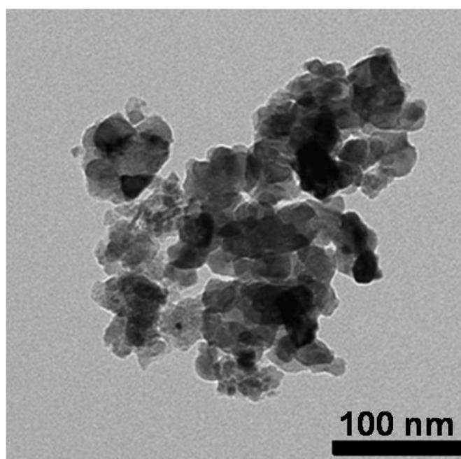
**Figure S5.** TEM image of particles synthesized in the absence of ammonium chloride at 900 °C.
