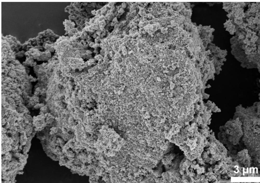
**Figure S1.** SEM image of the  $\text{Zn}_{1.7}\text{GeN}_{1.8}\text{O}$  particles synthesized with the urea pathway in the presence of ammonium chloride at 800 °C.
