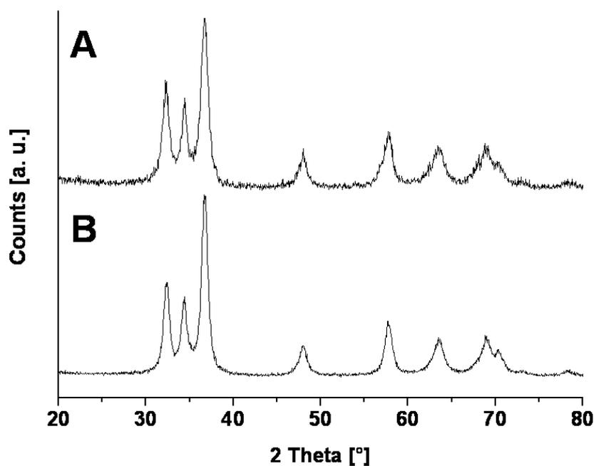
**Figure S10.** XRDs of the particles (A) after the catalytic measurements compared to the particles (B) before the catalytic measurements. Both show the typical reflexes of  $\text{Zn}_{1.7}\text{GeN}_{1.8}\text{O}$  (ICDD 00-024-1443).
