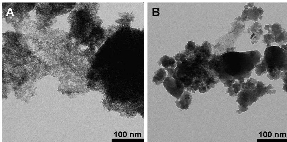
**Figure S8.** TEM images of the particles synthesized at 600 °C in the presence (A) and in the absence (B) of ammonium chloride. The presence of ammonium chloride leads to the formation of small and homogeneous particles.
