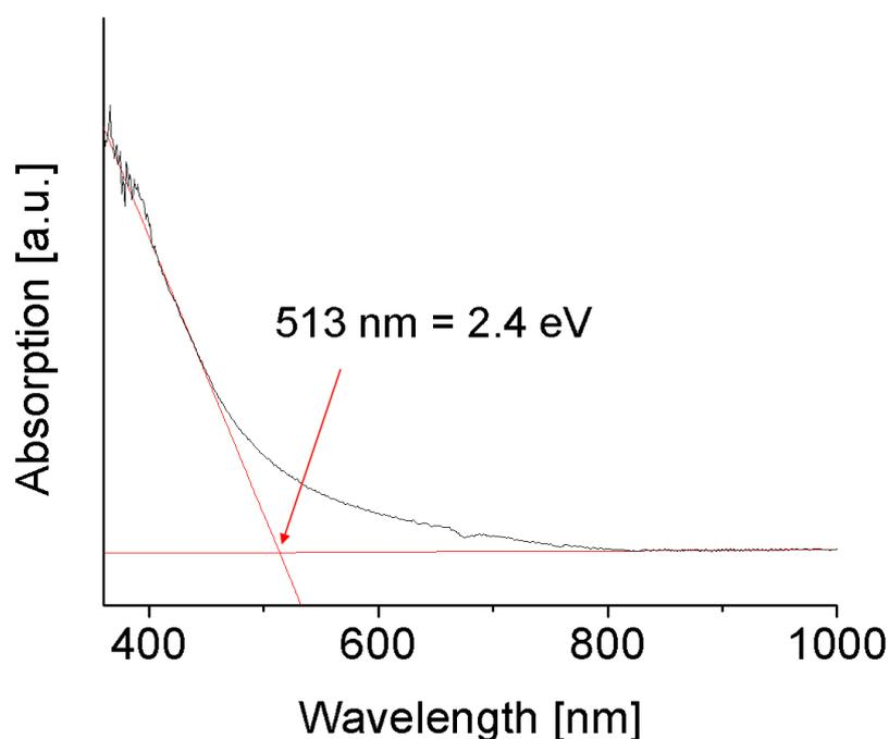
**Figure S2.** Absorption spectra of Zn<sub>1.7</sub>GeN<sub>1.8</sub>O. The band gap energy was determined, following a procedure described by A. E. Morales *et al.*<sup>[S1]</sup> Therefore two linear fits for the absorption slope ( $y = 16511.06 + 0.06x$ ) and for the background at lower energy ( $y = 31094.0 - 28.33x$ ) were done. The intersection of the two linear fits was determined to be at  $x = 513$  nm, which corresponds to a band gap energy of 2.4 eV.
