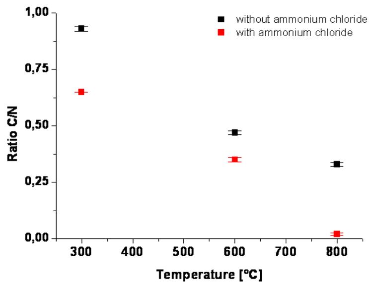
**Figure S9.** The amount of carbon and nitrogen in the samples synthesized at different temperatures was measured by elemental analysis. The plot illustrates the dependence of the ratio between C/N and the reaction temperature. The ratio of C/N was used as an indication for the progress of the reaction.
