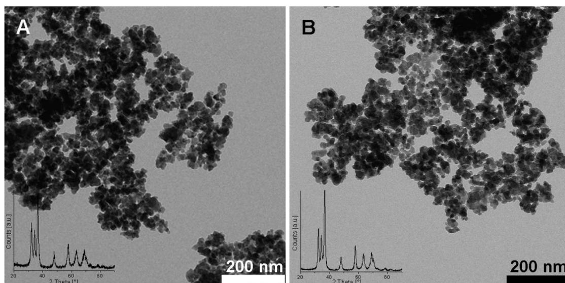
**Figure S4.** TEM images of Zn<sub>1.7</sub>GeN<sub>1.8</sub>O synthesized (A) with the recipe described in the experimental section and (B) with the tenfold up-scaled version of the recipe. The insets show the XRDs of the samples.
