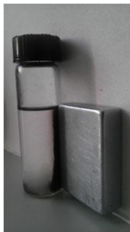
Figure S9. Photograph of magnetic separation of the Pt/ \gamma -Fe 2 O 3 -2 catalyst after hydrogenation.
