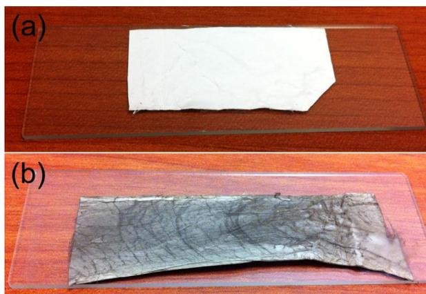
**Fig. S2.** The pictures of (a) electrospun PAN nanofibrous mat obtained using plate collector and (b) the above mat after 8-times PDA in-situ deposition under the same condition as that for the loose lump of PAN/Si nanofibers collected using water collector.
