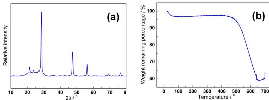
**Fig. S3.** (a) XRD pattern and (b) TGA profile of carbonized PAN/Si hybrid nanofibers (C-P/Si NFs). It is confirmed that the Si nanoparticles are in face-centered cubic crystalline form, and the content of Si in C-P/Si NFs is about 58.7 wt%.
