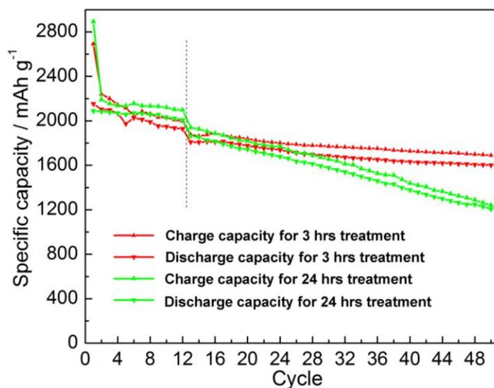
**Fig. S5.** Specific capacity of C-PDA/Si NFs and C-PDA/Si-24 NFs, which were prepared by treatment in DMF for 3 and 24 hrs, respectively, measured in cycling tests. It shows that the cyclability of C-PDA/Si NFs is better than that of C-PDA/Si-24 NFs, signifying the buffering effect of the remaining PAN-derived carbon around the Si nanoparticles.
