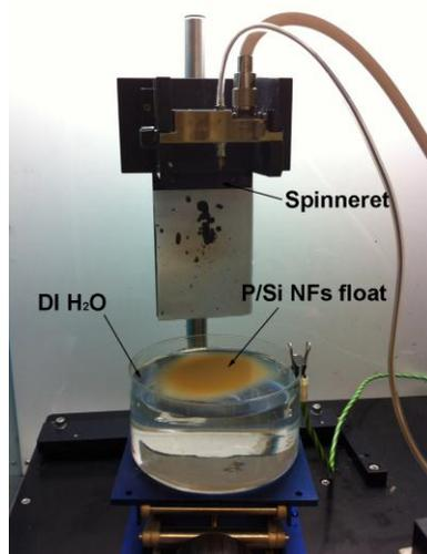
**Fig. S1.** The electrospinning setup with liquid collector.
