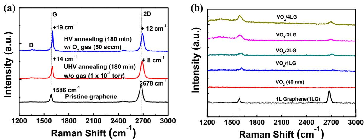
**Fig. S1** Raman spectra of graphene films according to (a) annealing processes, (b) VO<sub>2</sub> growth.
