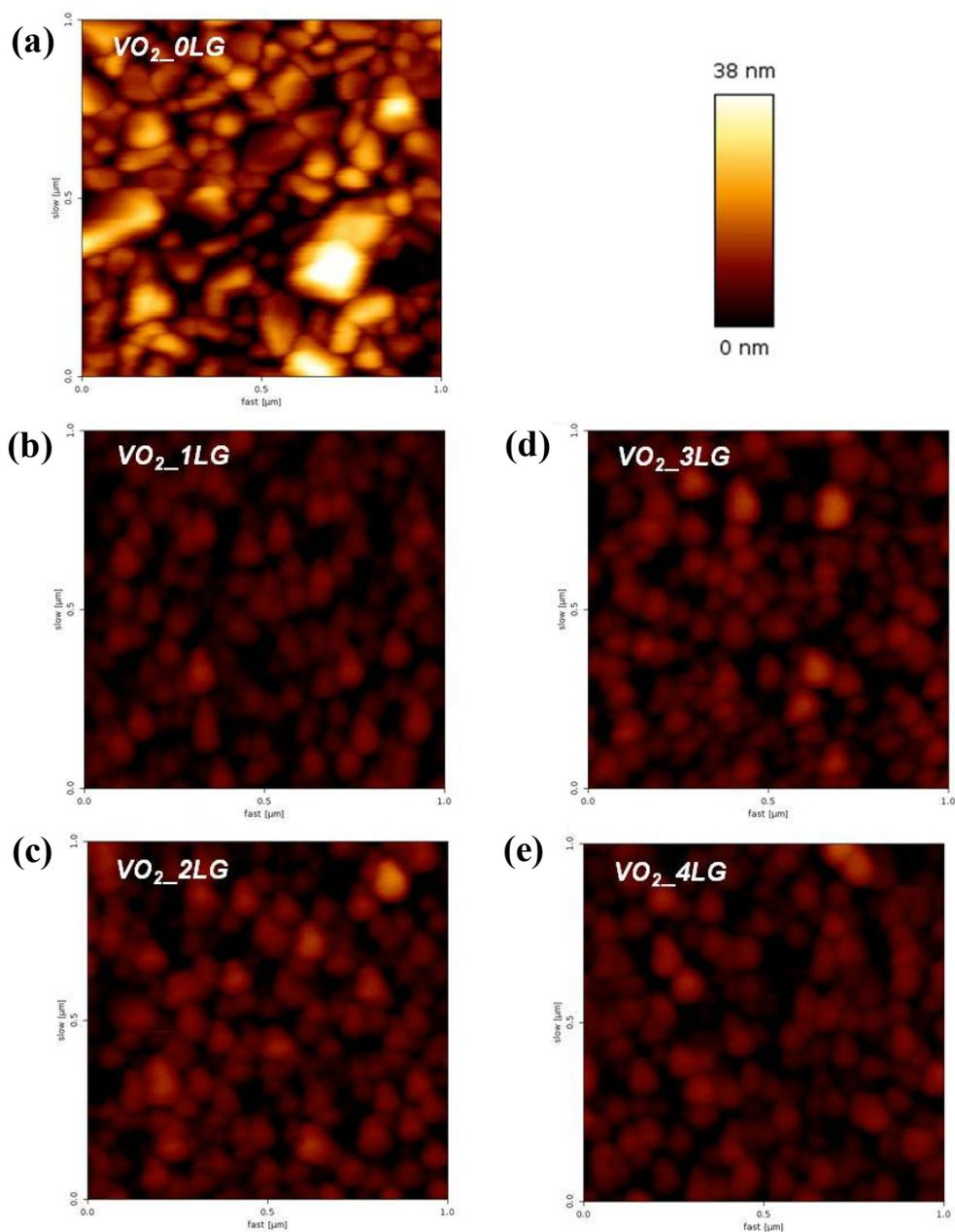
**Fig. S2** AFM images of the graphene-supported VO<sub>2</sub>. (VO<sub>2</sub> / x N layer/Sapphire)
