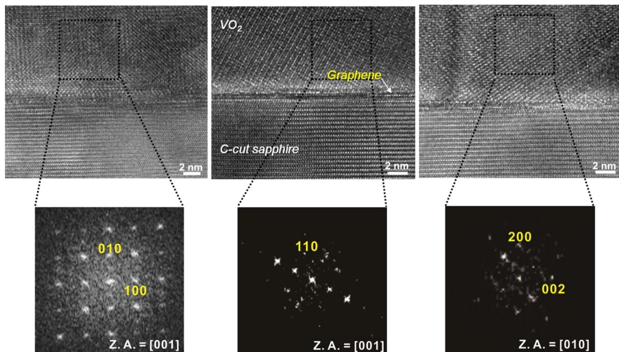
**Fig. S4.** High-resolution TEM images of the VO<sub>2</sub> films on graphene-supported sapphire substrate. (Various grains with different orientations could be observed)
