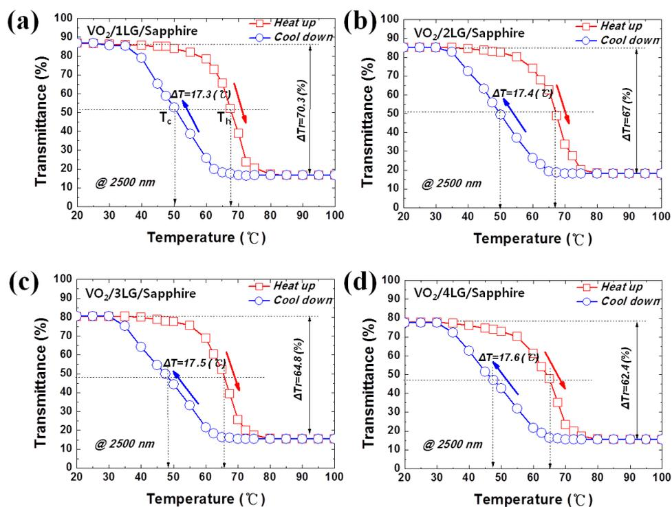
**Fig. S3** Temperature dependence transmittance of the graphene-supported VO<sub>2</sub>. (VO<sub>2</sub> / x N layer / Sapphire)
