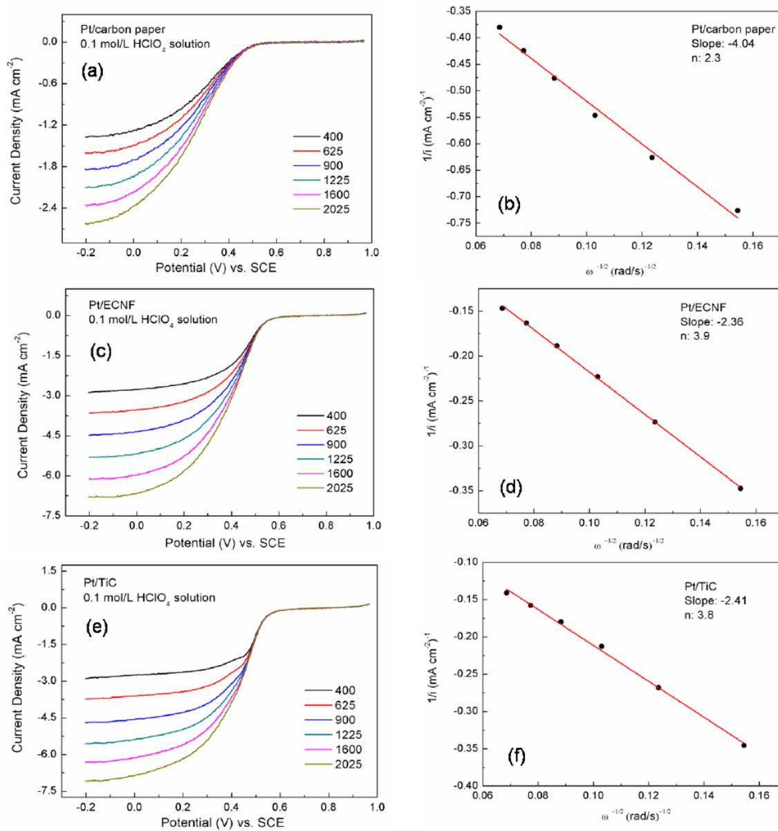
**Figure S3.** Polarization curves for the electrocatalytic systems of (a) Pt/carbon paper, (c) Pt/ECNF, and (e) Pt/TiC for ORR in 0.1 M HClO<sub>4</sub> scanned at 5 mV/s with different rotating rates, and the corresponding Koutecky-Levich plots of (b), (d), and (f).
