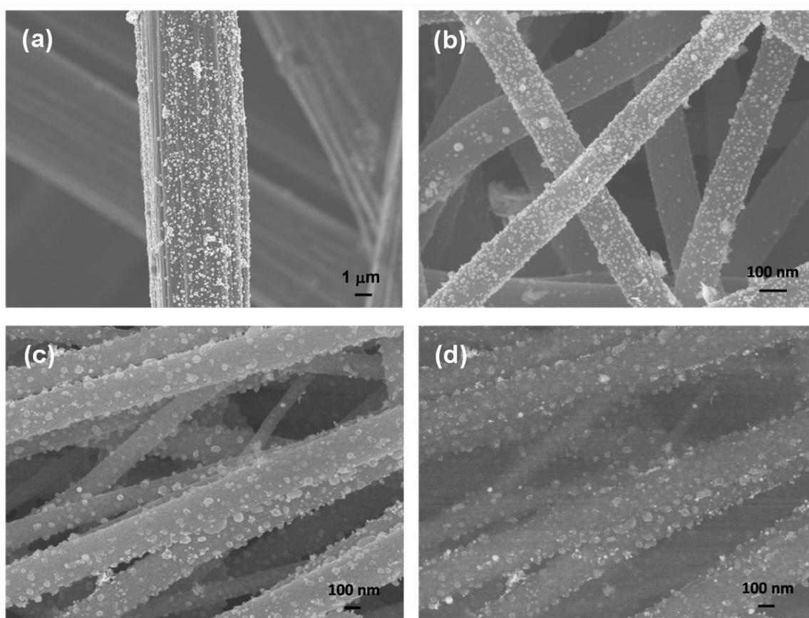
**Figure S1.** Representative SEM images of Pt NPs decorated on the surfaces of (a) carbon paper, (b) ECNF mat, and (c) TiC mat; (d) back-scattered electron image of (c).
