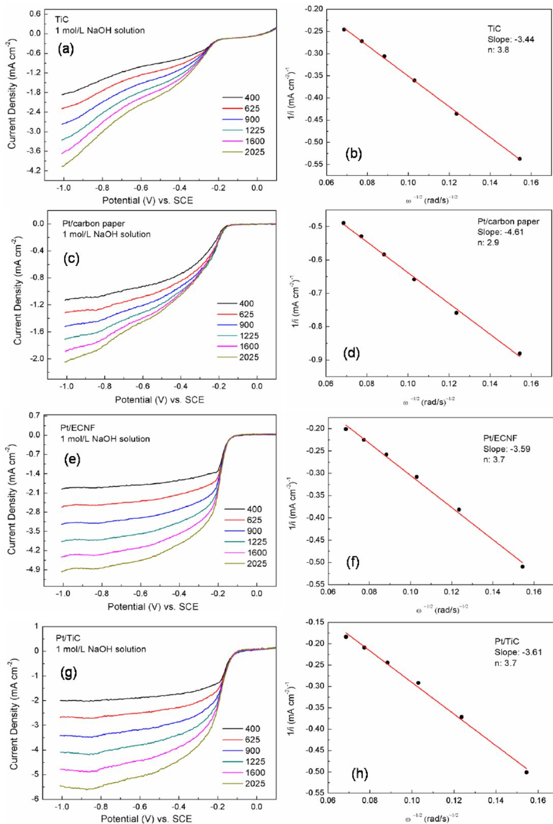
**Figure S4.** Polarization curves for the electrocatalytic systems of (a) TiC, (c) Pt/carbon paper, (e) Pt/ECNF, and (g) Pt/TiC for ORR in 1.0 M NaOH scanned at 5 mV/s with different rotating rates, and the corresponding Koutecky-Levich plots of (b), (d), (f), and (h).
