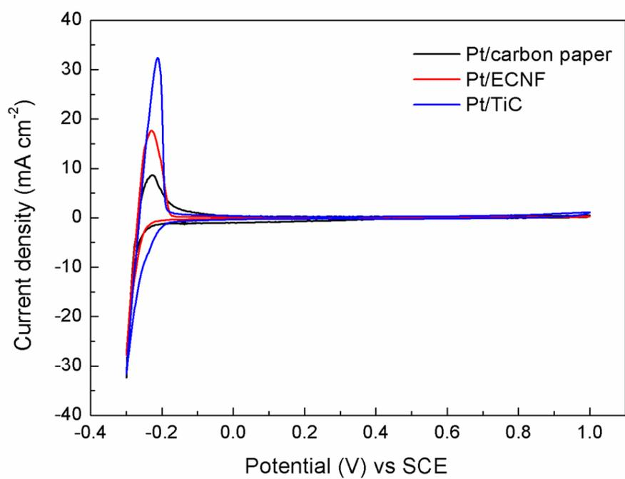
**Figure S2.** Cyclic voltammograms of the electrocatalytic systems of Pt/carbon paper, Pt/ECNF, and Pt/TiC in 0.5 M H<sub>2</sub>SO<sub>4</sub> solution at the scan rate of 50 mV/s.
