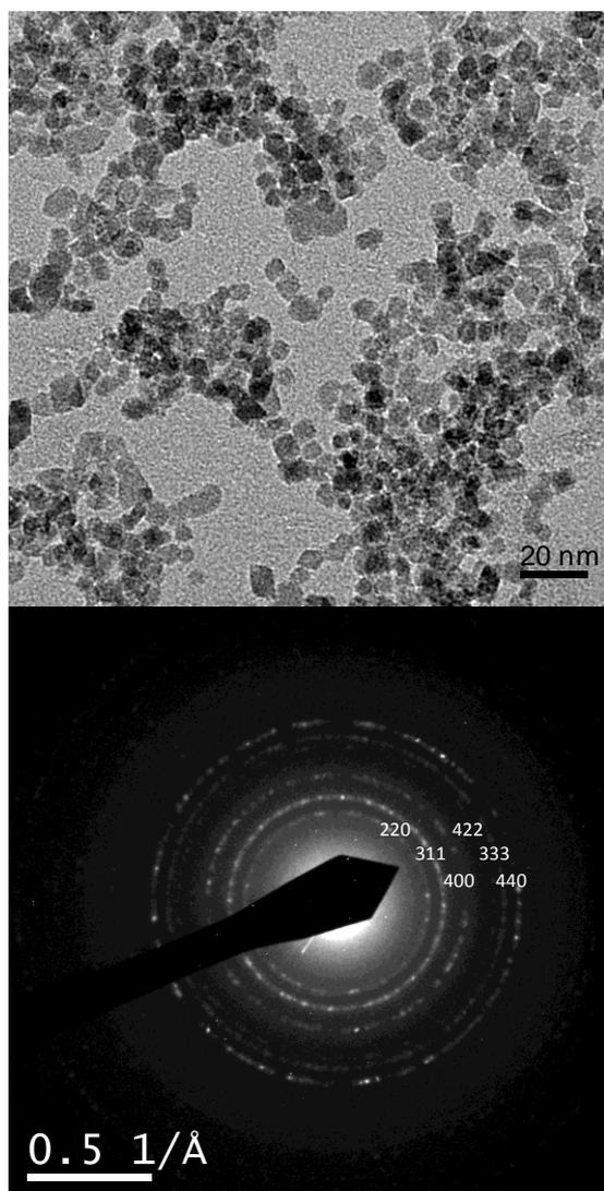
**Fig. S1.** TEM image of sample 250 °C and corresponding electron diffraction (ED) pattern showing spots/rings at distances expected for  $\text{CoAl}_2\text{O}_4$ .
