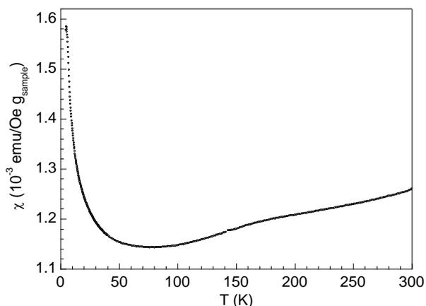
**Fig. S6.** Temperature dependence of the dc magnetic susceptibility of sample 200 °C recorded after ZFC procedure.
