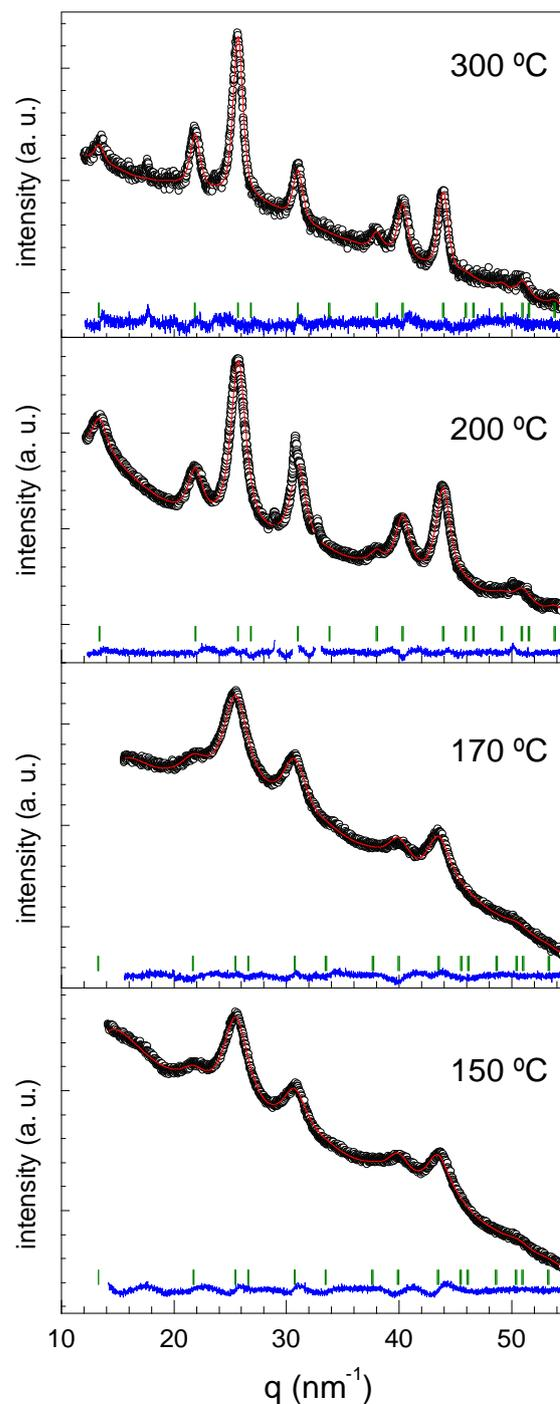
**Fig. S2.** XRD patterns of cobalt aluminium oxide samples produced at different temperatures. Continuous (red) line corresponds to Rietveld refinement of a spinel (space group  $Fd\bar{3}m$ ) using FullProf software<sup>S1</sup> considering mixed occupancy of tetrahedral and octahedral sites.
