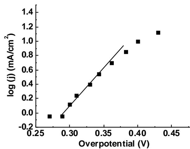
**Fig. S17** Tafel plot for *h*-Co@200. To get the Tafel plot, we measured steady-state current as a function of voltage with a dwell time of 5 min.
