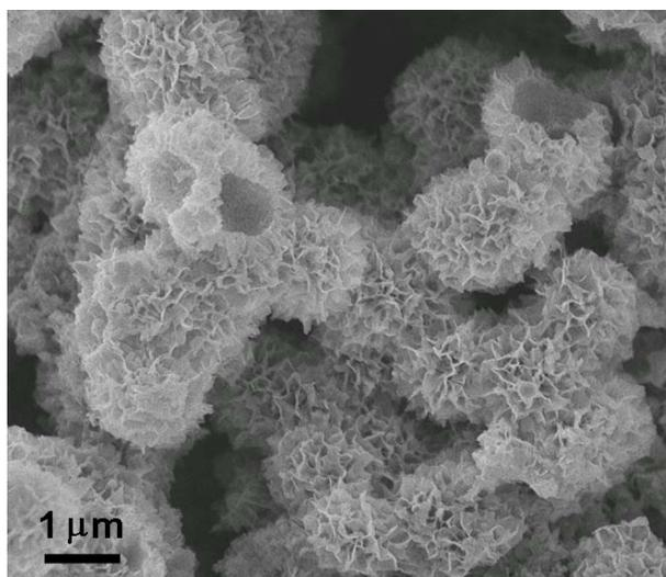
**Fig. S19** SEM image of *h*-Co@200 after photocatalytic O<sub>2</sub> evolution reaction.
