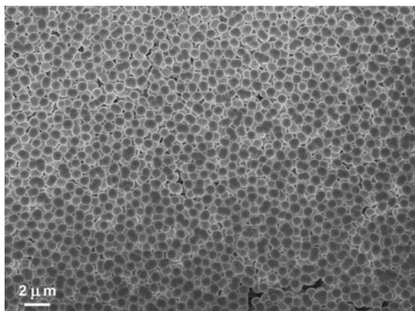
**Fig. S5** SEM image of the composite of the *s*-CoA sample.
