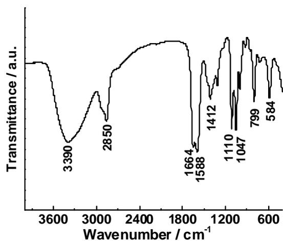
**Fig. S2** IR spectrum of the *s*-CoA sample. The broad IR absorption band at  $\sim 3390\text{ cm}^{-1}$  is attributed to hydrogen-bound hydroxyl groups, and the absorption band at  $\sim 2850\text{ cm}^{-1}$  is characteristic of the C-H stretching vibrations. In addition, all the bands located below  $2000\text{ cm}^{-1}$  are generally assigned to Co-O, C-C, C-C-O and C-O-Co groups. Similar IR results were also observed previously for other metal alkoxides.<sup>[S1-2]</sup>
