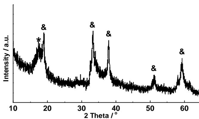
**Fig. S7** XRD pattern of the *h*-CoOH sample. Fig. S7 reveals that *h*-CoOH possibly contains both  $\beta$ -Co(OH)<sub>2</sub> (which is marked by “&”) and cobalt carbonate hydroxide (Co(CO<sub>3</sub>)<sub>0.5</sub>(OH)·0.11H<sub>2</sub>O, which is marked by “\*”).
