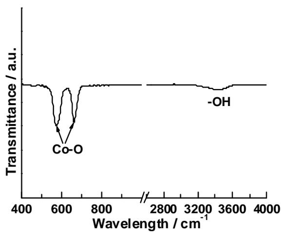
**Fig. S11** IR spectrum of *h*-Co@200. The IR spectrum of *h*-Co@200 is in agreement with that of spinel  $\text{Co}_3\text{O}_4$ .<sup>[S6]</sup>
