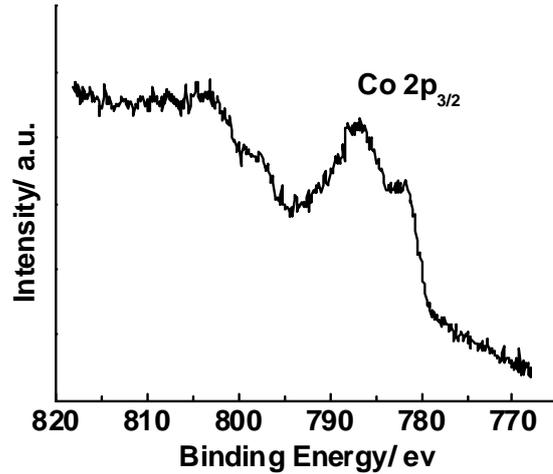
**Fig. S3** Co 2p electron XPS spectrum for *s*-CoA spheres. Two  $2P_{3/2}$  XPS peaks were detected at 786.6 and 802.8 eV, indicating the presence of Co (II) species.<sup>[S7]</sup>
