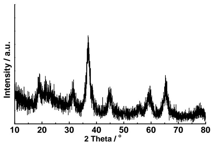
**Fig. S18** XRD pattern of *h*-Co@200 after photocatalytic O<sub>2</sub> evolution reaction.
