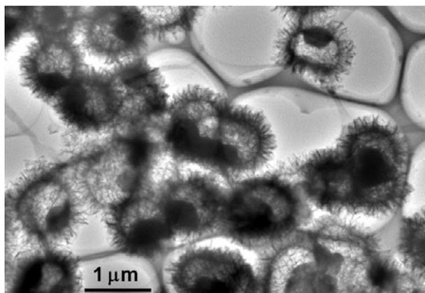
**Fig. S10** TEM image of the product obtained after hydrothermal treatment of *s*-CoA for 60 min.
