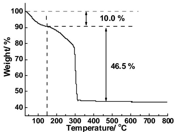
**Fig. S4** TG curve measured in air for the *s*-CoA sample. TG analysis of *s*-CoA was carried out in air from 25 to 800 °C. Before 150 °C, the weight loss of 10.0% can be attributed to evaporation of the absorbed organic residues and water species on the *s*-CoA surface. The *s*-CoA completely decomposed at around 300 °C with a total weight loss of ~46.5 %. From the weight loss values it is estimated that the empirical composition of *s*-CoA is  $C_3H_6O_3Co$ .
