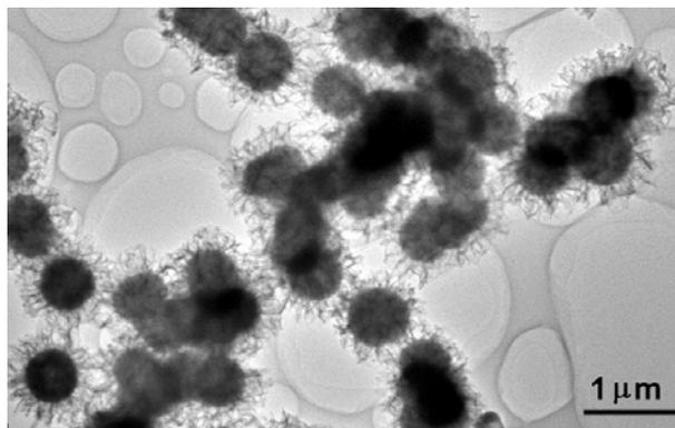
**Fig. S9** TEM image of the product obtained after hydrothermal treatment of *s*-CoA for 15 min.
