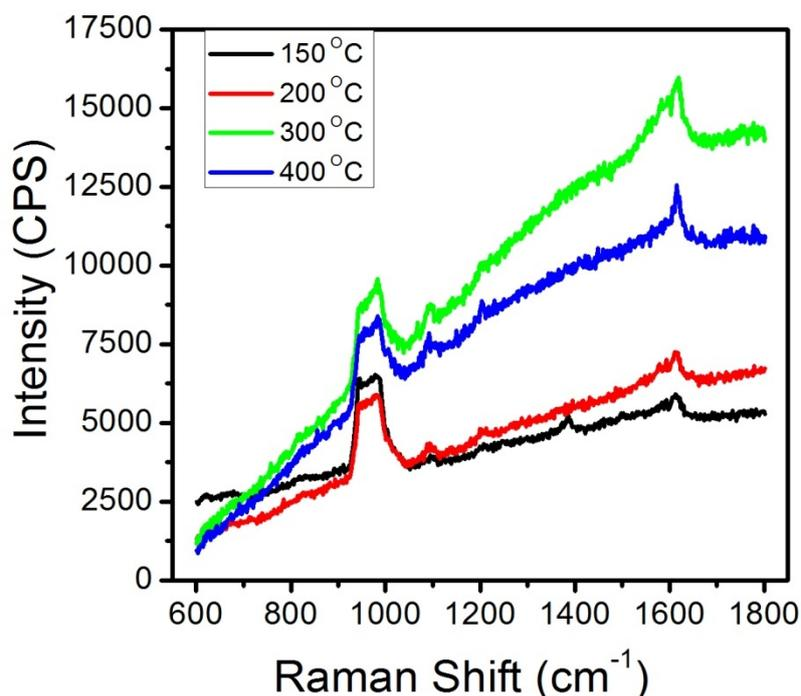
Fig. S3 SERS spectra with 532-nm excitation of the 4-MPy modified gold nanoisland structures annealed at different temperatures.
