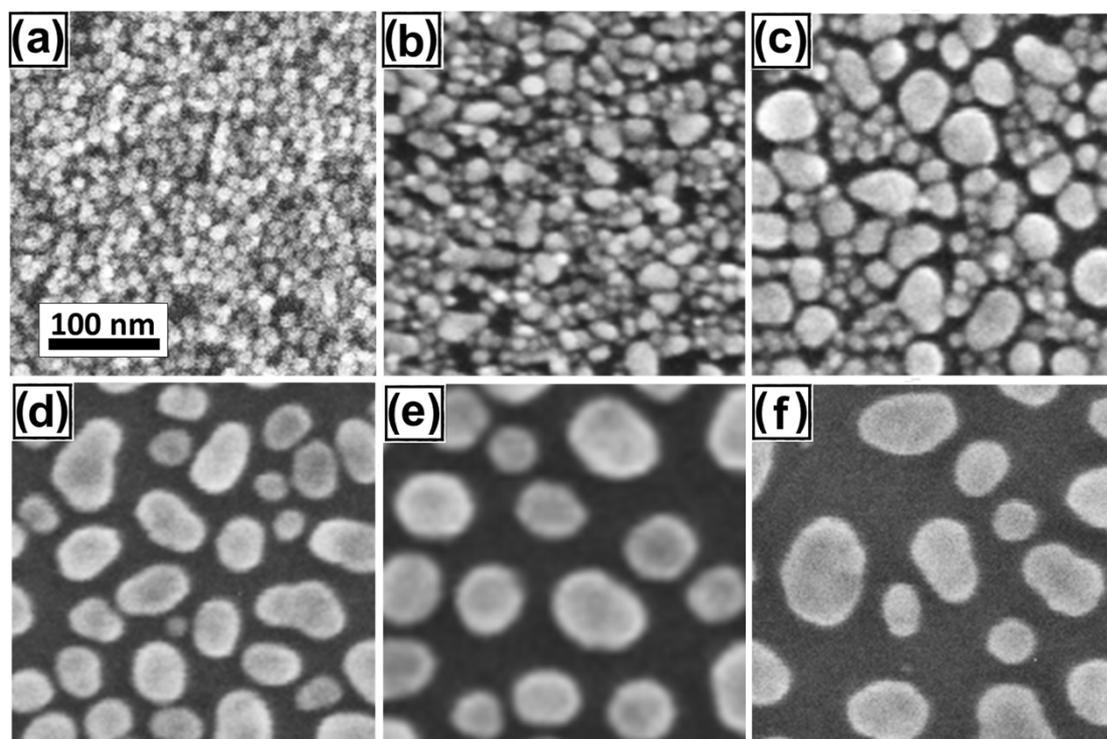
Fig. S1 Enlarged SEM images of the gold nano-island structures obtained at annealing temperatures of: (a) 140 °C, (b) 150 °C, (c) 200 °C, (d) 300 °C, (e) 400 °C, and (f) 500 °C.
