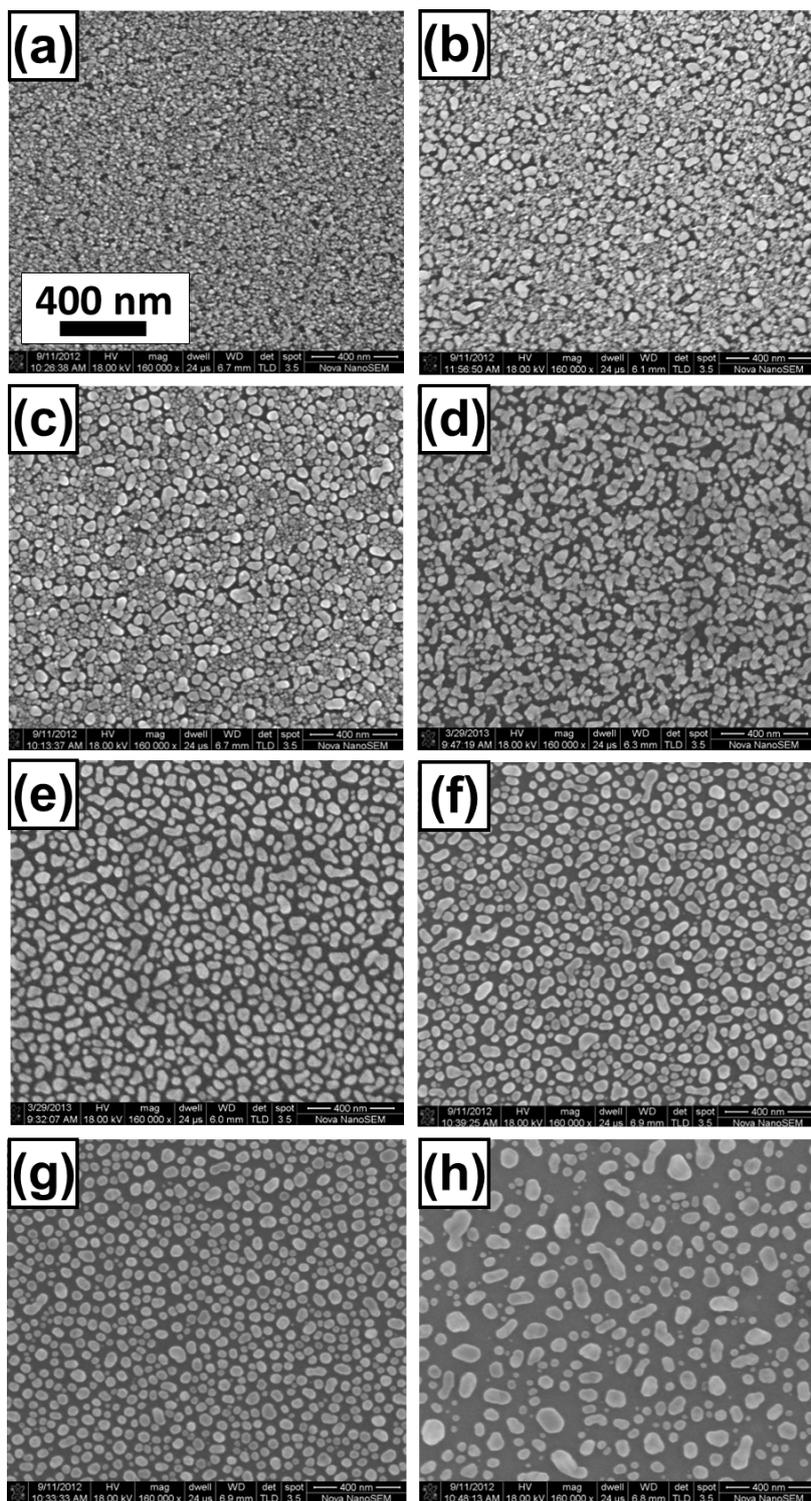
Fig. S2 SEM images of the gold nano-island structures obtained at annealing temperatures of: (a) 150 °C, (b) 180 °C, (c) 200 °C, (d) 220 °C, (e) 250 °C, (f) 300 °C, (g) 400 °C, and (h) 500 °C.
