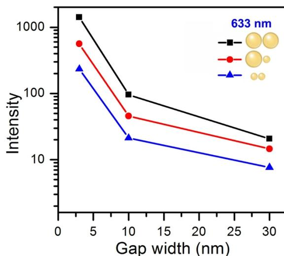
Figure S6 Variation of the intensity of electric field with the gap width for three combinations between the two kinds of gold nanoparticles ( $D=40$  and 70 nm) for an excitation laser at 633 nm with the same polarization as shown in Fig. S5.
