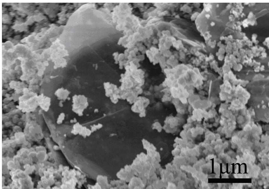
**Fig. S1** SEM image of  $\text{Cu}_x\text{O}$ /multilayer graphene composite using EG as carbon resource
