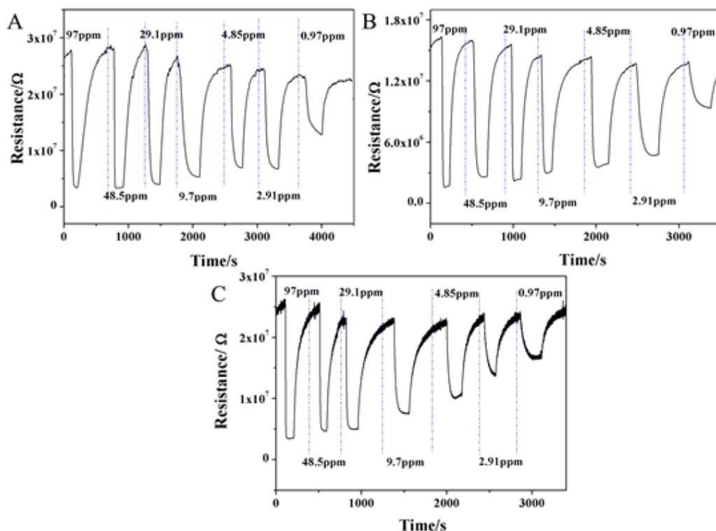
**Fig. S12** The dynamic response- recovery curve of the CuMGC2 sensor to 97 ppm~97 ppb NO<sub>x</sub> at room temperature in the different RH (A) 41%, (B) 62 % and (C) 80 %
