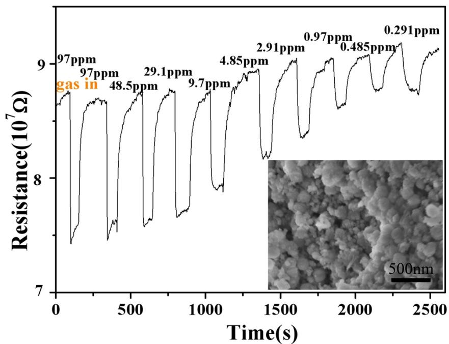
Fig. S9 Typical response curves of the  $\text{Cu}_x\text{O}$  sensor to 97~0.97 ppm  $\text{NO}_x$  at room temperature, the inset SEM image of the prepared  $\text{Cu}_x\text{O}$
