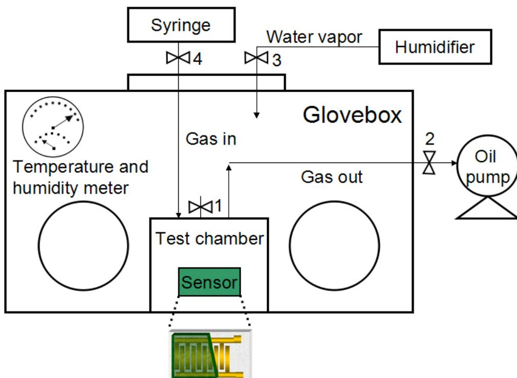
**Fig. S4** A diagram of the gas delivery system for the gas sensing process
