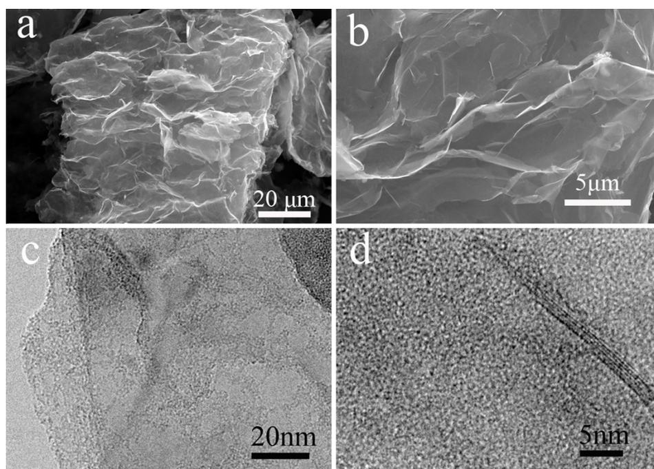
**Fig. S5** (a, b) SEM images of activated expanded graphite (aEG) showing the accordion-like structure; (c, d) TEM images of aEG with many pores on the its surface
