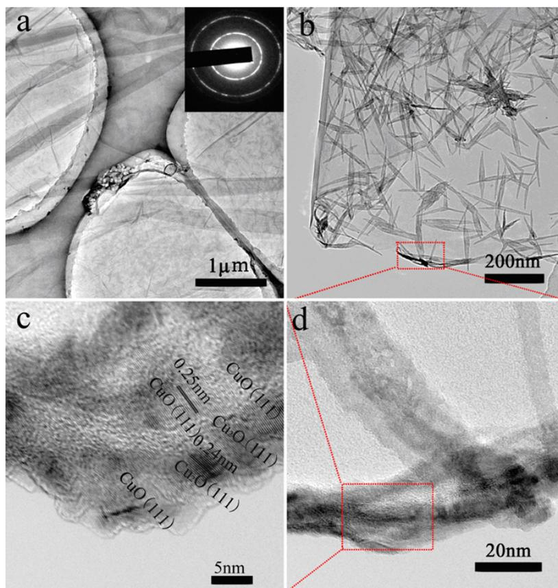
**Fig. S2** (a) TEM image of GO, the inset shows the SAED pattern; (b) Representative TEM image of  $\text{Cu}_x\text{O}/\text{RGO}$ ; (c) HRTEM image of part of  $\text{Cu}_x\text{O}/\text{RGO}$ ; (d) TEM image of  $\text{Cu}_x\text{O}/\text{RGO}$
