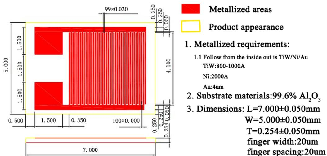
**Fig. S3** The image of interdigitated gold electrode and its parameters.
