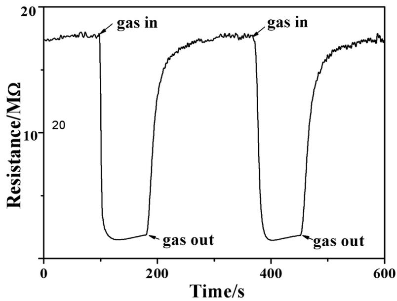
Fig. S11 Typical response curves of the CuGNC2 sensor to 48.5 ppm NO<sub>x</sub> at room temperature
