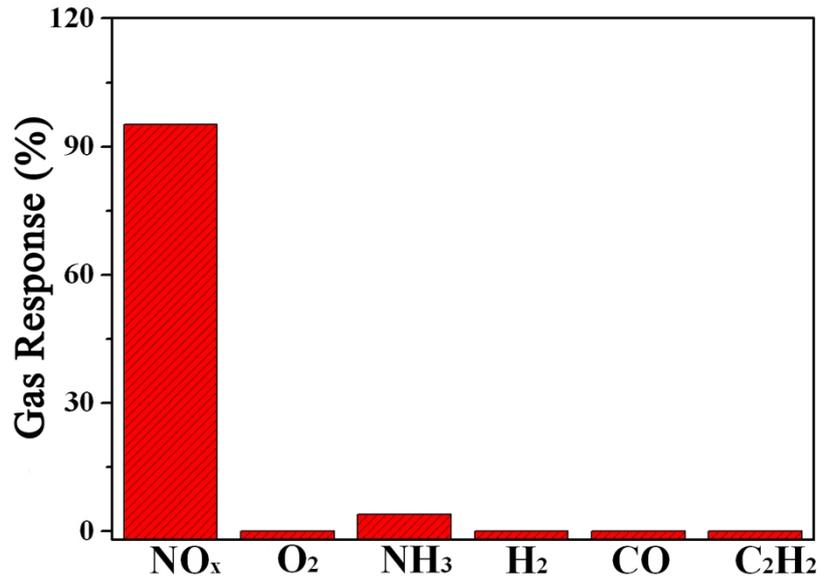
Fig. S10 Response of the CuGNC2 sensor to 97.1 ppm different gases at room temperature in air
