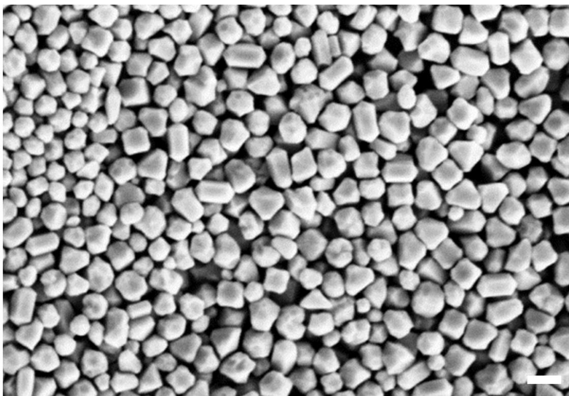
**Figure S10.** SEM image of Pd nanoparticles synthesized without using KI. Other conditions are the same as making 295 nm rods. Scale bar: 200 nm.
