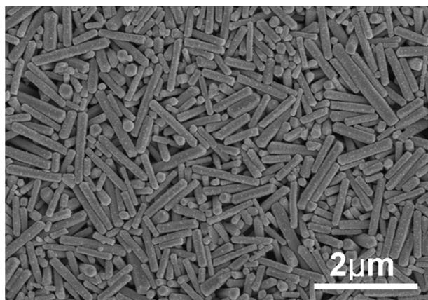
**Fig. S1.** SEM image of Ag<sub>2</sub>CO<sub>3</sub> nanorods.
