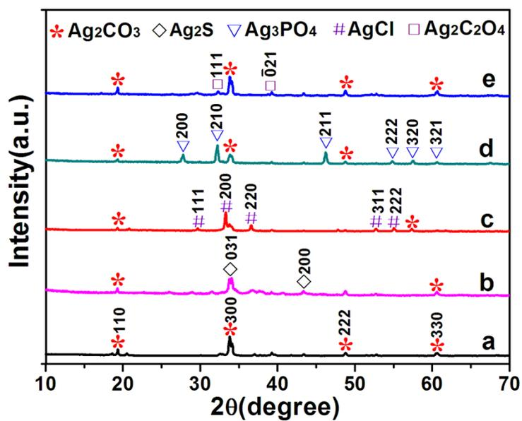
**Fig. S4.** XRD patterns of (a) the as-prepared pure Ag<sub>2</sub>CO<sub>3</sub> nanorods and different Ag<sub>2</sub>CO<sub>3</sub>-Ag<sub>n</sub>X yolk-shell nanostructures: (b)Ag<sub>2</sub>CO<sub>3</sub>-Ag<sub>2</sub>S; (c)Ag<sub>2</sub>CO<sub>3</sub>-AgCl; (d)Ag<sub>2</sub>CO<sub>3</sub>-Ag<sub>3</sub>PO<sub>4</sub>; (e)Ag<sub>2</sub>CO<sub>3</sub>-Ag<sub>2</sub>C<sub>2</sub>O<sub>4</sub>.
