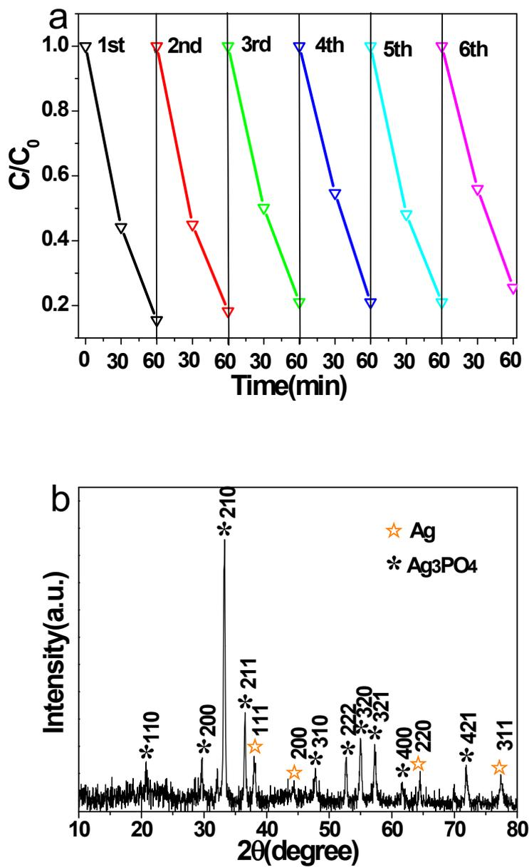
**Fig. S7.** (a) 6 cycles of degradation of RhB using  $Ag_3PO_4$  NTs as photocatalyst; (b) XRD pattern of the  $Ag_3PO_4$  NTs after six cycles of the photocatalytic test.
