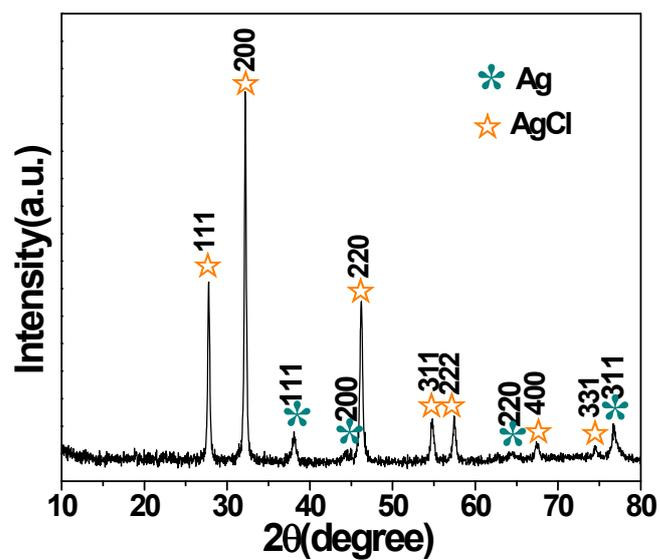
**Fig. S6.** XRD pattern of the  $\text{AgCl}$  NTs after six cycles of the photocatalytic test.
