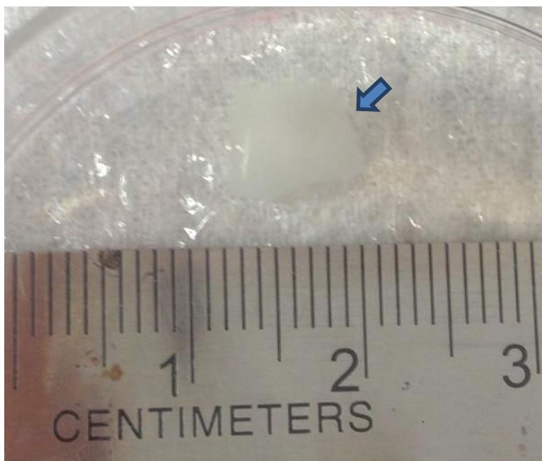
Figure S3. Digital picture of a freely suspended PVDF nanomembrane (5 x 5 mm) floating on a water surface.
