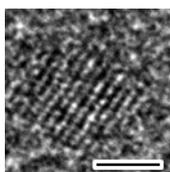
**Figure S1:** HRTEM micrograph of PbS NCs (scale bar = 2nm).
