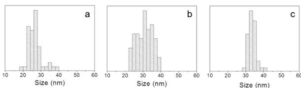
**Figure S2:** Size distribution histograms of PbS@SiO<sub>2</sub> samples prepared with 700  $\mu$ L of Igepal, 400  $\mu$ L of ammonia, 30  $\mu$ L of TEOS achieving a PbS NC concentration of  $6.1 \cdot 10^{-6}$  M (a) and  $9.5 \cdot 10^{-6}$  M (b). Size distribution histogram of PbS@SiO<sub>2</sub> sample prepared with 700  $\mu$ L of Igepal, 400  $\mu$ L of ammonia, 80  $\mu$ L of TEOS, achieving a PbS NC concentration of  $6.1 \cdot 10^{-6}$  M (c).
