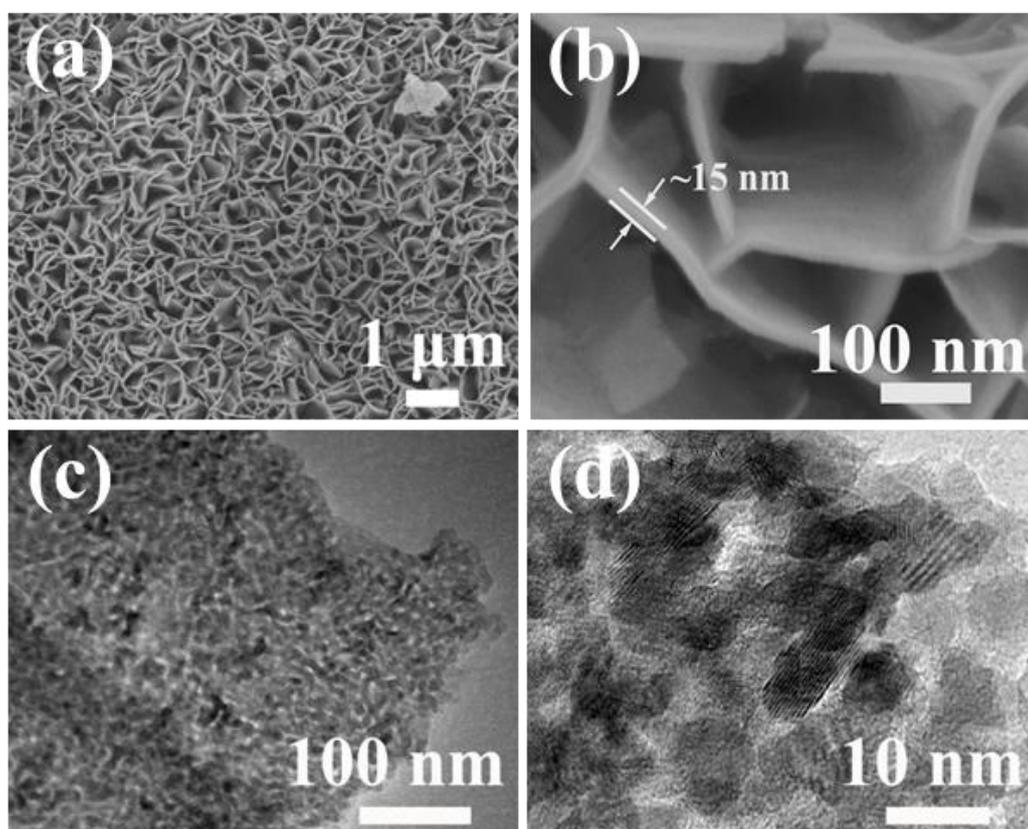
Fig. S3. SEM (a, b) and TEM (c, d) images of the Co<sub>3</sub>O<sub>4</sub> nanosheets growing directly on Ni foam for comparison.
