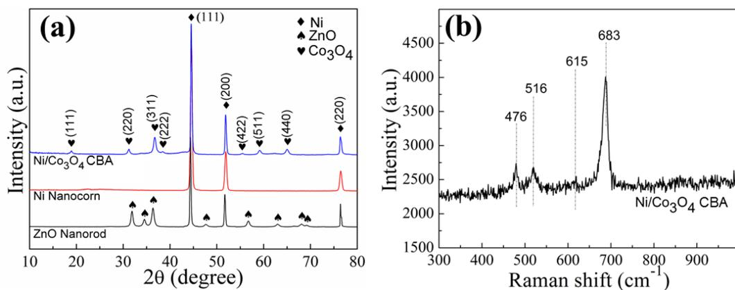
Fig. S2. (a) XRD patterns of the ZnO nanorod, hollow Ni Nanocorn and Ni/Co<sub>3</sub>O<sub>4</sub> CBAs on nickel foam. (b) Raman spectra of Ni/Co<sub>3</sub>O<sub>4</sub> CBAs.
