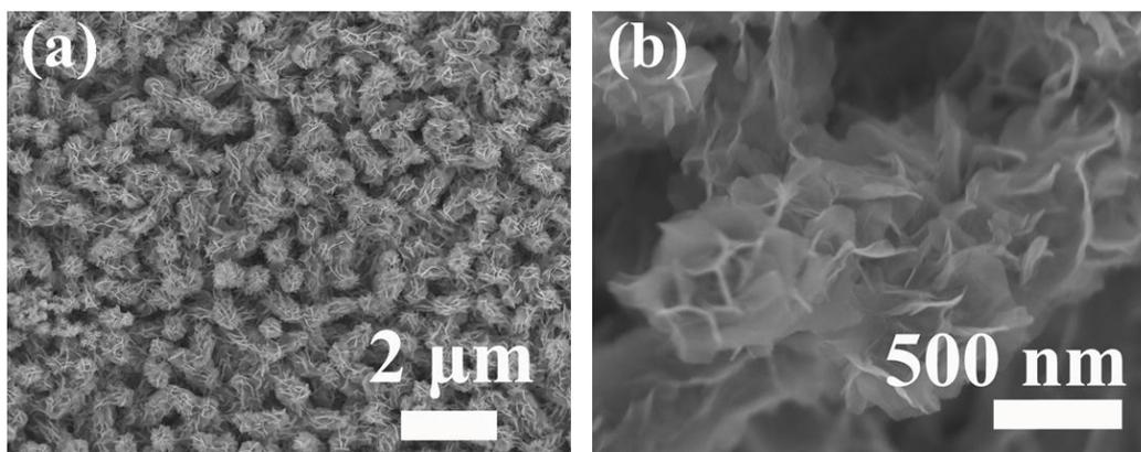
Fig. S5. SEM images of the  $\text{Ni}/\text{Co}_3\text{O}_4$  CBAs after cycling for 10000 cycles.
