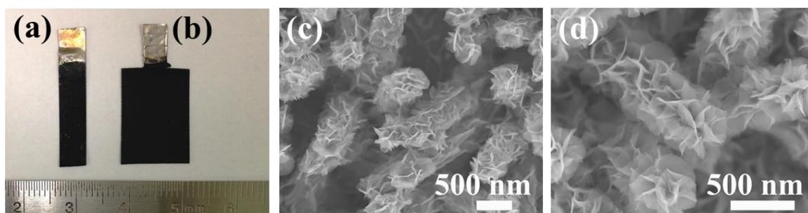
Fig. S1. Photographs and SEM images of Ni/Co<sub>3</sub>O<sub>4</sub> CBAs grown on different substrates. (a, c) Ti foil and (b, d) stainless steel foil substrates.
