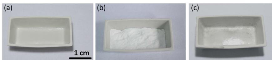
**Fig. S1** (a) The empty rectangular porcelain boat. (b) The melamine power undergoes the solvothermal treatment at 140 °C as typical experiment in the porcelain boat; (c) The above mentioned melamine power after thermally annealing process at 800 °C. After thermally annealing process, noting left but an empty rectangular porcelain boat, indicating the sublimation process was dominant under high temperature.
