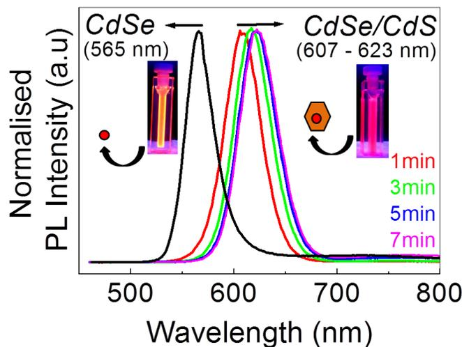
**Fig. S6.** Red shifting of the PL peak of the 2D core/shell NCs with growth time with respect to the starting CdSe core.
