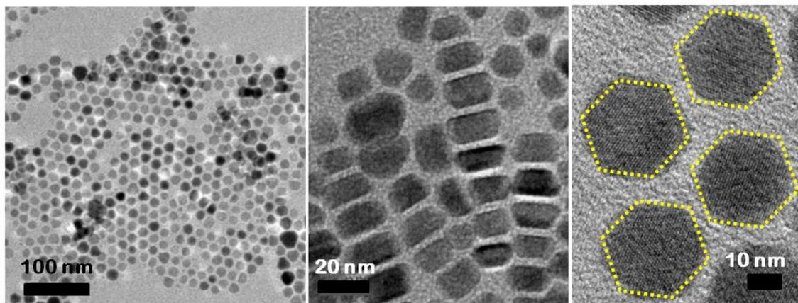
**Fig. S1.** Additional TEM and HRTEM images of CdSe/CdS core@shell 2D nanoheterostructure samples. The left panel is for low magnification image, middle panel for self-assembled particles lying on the edges and the right panel for HRTEM image.
