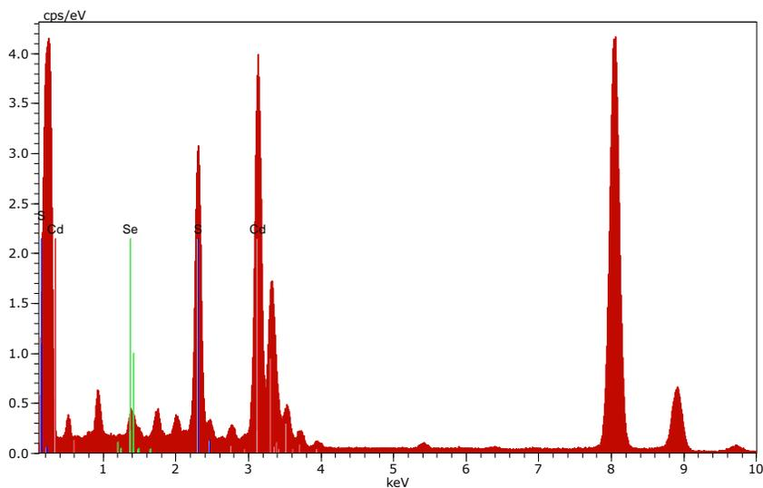
**Fig. S2.** EDAX of core@Shell from CdSe-A showing the presence of Cd, Se and S.
