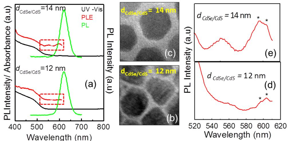
**Fig. S5.** Comparison of optical absorption, PLE and PL spectra of 2D CdSe/CdS nanoheterostructures with increasing shell size (growth). (a) UV-Vis, PLE, PL of two CdSe/CdS core/shell samples (b,c) TEM images of the corresponding samples. (d,e) Magnified PLE spectra in the range 520-620 nm, taken from the selected area in panel ‘a’.
