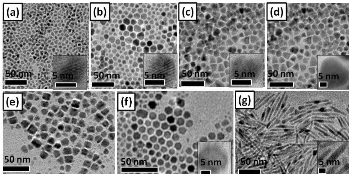
**Fig. S3.** Control reaction TEM images from table 1. Here panel (a) corresponds to reaction serial No 1, (b) to 2, (c) to 3, (d) to no CdO, (e) to no CdSe core, (f) to No S and (g) corresponds to reaction 7 for nanorods, respectively.
